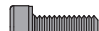
Z543 Cap Head Screw M3x10mm Inbusschraube M3x10mm Vis tête cylindrique M3x10mm キャップネジ M3x10mm
