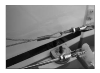
Adjust the pull-pull cables in the rigging couplers to center the rudder and remove slack from the cables. Use a ruler to check the alignment of the rudder to the fin while making the adjustments.
