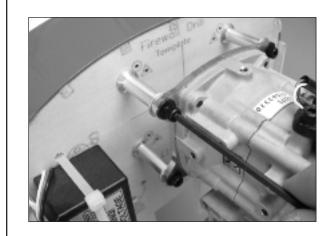
Use a 3mm hex wrench to reinstall the carburetor isolator block.
