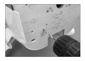
Locate a 28mm aluminum standoff,  $8-32 \times 1 \frac{1}{2-inch}$  socket head cap screw, #8 washer and #8 blind nut. Place the washer and standoff on the cap screw.
