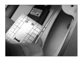
Use pliers to make a 90-degree downward bend in the pushrod at the mark made in Step 17. Trim the wire to a length of approximately 5/16-inch.
