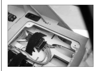
Use small cable ties to organize the servo leads in the radio compartment.
