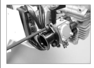
☐ **Step 15**Reattach the ball link connector to the throttle arm.
