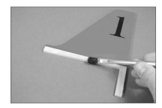
$\Box$  5. Fit the fin into the fuselage. Use a paper towel and rubbing alcohol to remove any excess epoxy that oozes out when the fin is installed.
