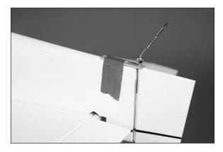
$\Box$  23. Use a pin vise and 1/16-inch (1.5mm) drill bit to drill the two holes in the fuselage for the mounting screws.
