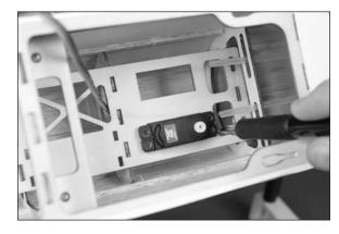
$\Box$  5. Remove the servo from the fuselage. Use a pin vise and 1/16-inch (1.5mm) drill bit to drill the holes for the servo mounting screws.
