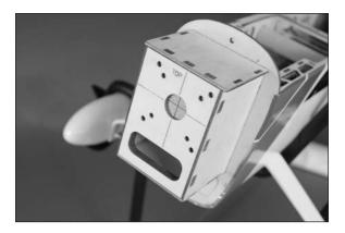
$\Box$  2. Use a drill and 1/8-inch (3mm) drill bit to drill the four holes for mounting the engine. Use the inner set of holes for the Power 25, the outer set of holes for the Power 32.
