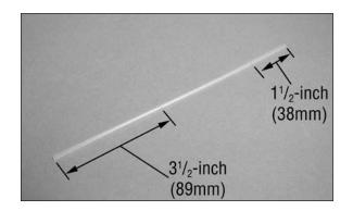
$\Box$  14. Slide the tube into the fuselage with the 1<sup>1</sup>/<sub>2</sub>-inch (38mm) first. Note the position of the tube inside the fuselage as it passes through the formers. Position the tube so 3<sup>1</sup>/<sub>2</sub>-inch (89mm) of the tube is exposed forward of the fuselage as shown.
