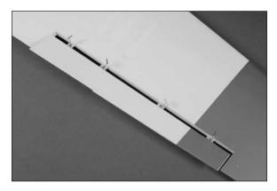
□□ 6. Remove the T-pins from the hinges. Make sure the aileron is pressed tightly against the wing panel to eliminate any hinge gap. Check that the ends of the aileron have an equal gap and are centered in the opening for the aileron in the wing panel.
