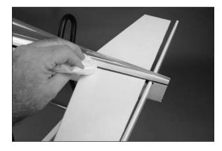
□ 15. Before the epoxy can cure, make sure to check the alignment of the stabilizer as described in steps 7 through 9. It is very important the stabilizer is positioned correctly before the epoxy begins to cure, as it will be difficult to readjust its position after the epoxy has cured. Do not proceed until the epoxy has fully cured.
