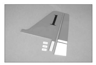
$\Box$  2. Test fit the fin at the rear of the fuselage. Slide the fin as far forward as possible. Use a felt-tipped pen to transfer the outline of the fuselage to the fin.
