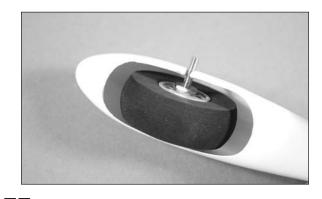
□□ 9. Insert the threaded portion of the axle through the larger hole of the landing gear. Use a 10mm open-end wrench and 7mm nut driver to tighten the 4mm nut that secures the axle. Leave the nut a little loose so the wheel pant can be moved easily for adjustment.
