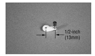
$\Box$  9. Use the transmitter to center the throttle servo. Center the throttle stick and trim, then install the servo horn as shown. This will provide equal throw for both full- and closed-throttle. Use a #1 Phillips screwdriver and the screw removed from the servo to secure the horn on the servo.
