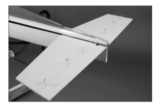
$\Box$  19. Remove the T-pins from the hinges. Make sure the elevator is pressed tightly against the stabilizer to eliminate any hinge gap. Check that the tips of the elevator and stabilizer are aligned.
