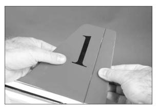
$\Box$  21. Flex the rudder through its range of motion a number of times to break in the hinges. This will reduce the load on the servo for those first flights.
