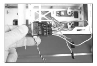
$\Box$  3. Use hook and loop tape to secure the receiver in the fuselage. Make sure to route the leads so they don't interfere with the operation of the servos.
