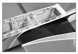
**Note**: The wing does not need to be secured to the fuselage at this time. It is only being installed so the position of the stabilizer can be adjusted.
