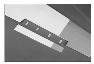
$\Box$  2. Use a pin vise and 1/16-inch (1.5mm) drill bit to drill a hole in the center of each hinge slot. This will provide a tunnel for the CA to wick into, providing a better bond between the wood and hinge when they are glued in position. Prepare both the aileron and wing panel at this time.
