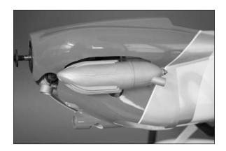
$\Box$  7. Attach the propeller and spinner to the engine. Follow the instructions provided with the engine to make sure the propeller is secure.
