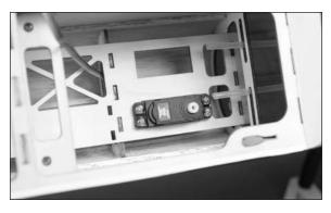
□□ 9. Prepare the servo horn by enlarging the hole in the arm that is 3/8-inch (9.5mm) from the center of the servo horn using a pin vise and 5/64-inch (2mm) drill bit. Use side cutters to remove any other arms from the horn so they don't interfere with the operation of the servo.
