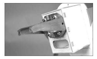
$\Box$  10. Place the engine between the mount and slide the nylon mounting beams tight against the engine case. Slide the engine and mount as far to the left as possible, as this will center the propeller shaft with the cowling when it is installed.
