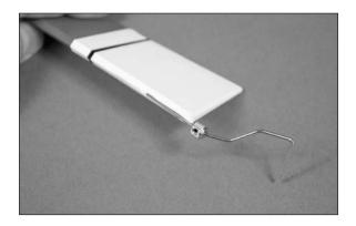
$\Box$  11. Remove the tail gear wire from the rudder. Use medium grit sandpaper to roughen the tail gear wire where it contacts the rudder.
