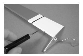
$\Box$  15. Place a T-pin in the center of the three hinges removed in step 1. This will center the hinges evenly in the rudder and fin.
