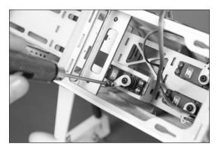
□ 18. Check the operation of the throttle to make sure the carburetor moves from open to closed. You may need to make adjustments at the radio so the servo does not bind at either extreme.
