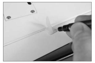
$\square$  3. Use a pin vise and a 5/64-inch (2mm) drill bit to drill the holes for the control horn mounting screws.
