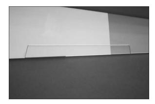
$\Box$  7. Saturate each hinge using thin CA on both the top and bottom of the hinge. Allow the CA to fully cure before proceeding.
