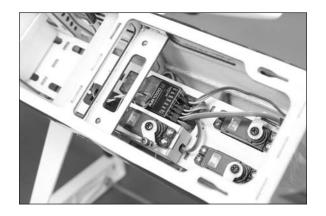
$\Box$  4. Mount the remote receiver in the fuselage away from the main receiver using hook and loop tape. Make sure to orient the antenna on the remote receiver in a different direction than those on the main receiver for the best reception from your radio system.
