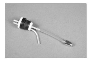
$\Box$  8. Insert the stopper assembly into the fuel tank. Make sure the vent line faces to the top of the tank as shown. Note that the hole in the tank is off-center. The hole for the stopper will be closer to the bottom of the tank.
