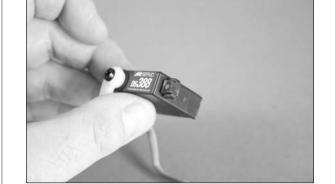
$\Box$  2. Use a pin vise and 5/64-inch drill bit to enlarge the hole in the servo arm that is 1/2-inch (13mm) from the center of the horn as shown.
