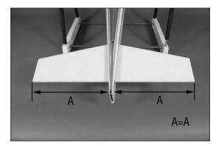
$\square$  8. Measure from each wing tip to each stabilizer tip. Position the stabilizer so both measurements are equal as shown.
