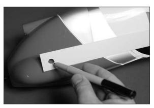
$\Box$  3. Use hobby scissors and a rotary tool with a sanding drum to remove the material necessary to fit the cowl over the engine. Work slowly, removing only small amounts from the cowl at a time. Test fit the cowling periodically to make sure it is fitting properly. Create a small opening for the muffler at this time as well.
