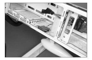
$\Box$  4. Secure the battery in the fuselage using hook and loop straps. Use a piece of hook and loop tape along the bottom of the battery to keep it from sliding on the battery tray.
