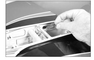
$\Box$  6. Use two 3mm x 10mm socket head screws and two 3mm washers to secure the wings to the fuselage. Use a 2.5mm hex wrench to tighten the bolts securing the wing.
