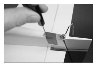
□ 24. Remove the tape and swing the bracket to the side. Thread a 2mm x 8mm self-tapping screw into each hole to cut threads in the surrounding wood using a #1 Phillips screwdriver. Remove the screw before proceeding to the next step.
