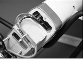
Note: Drill a 1/8-inch (3mm) hole in the bottom of the motor box and use a tie wrap (not included) to secure the wires so they don't interfere with the operation of the motor.
