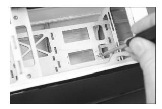
□□ 7. Apply 2–3 drops of thin CA in each hole to harden the surrounding wood. This will help prevent the screws from vibrating loose.
