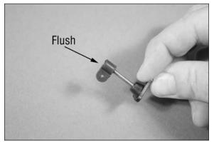
$\Box$  2. Prepare the rudder control horn by threading the control horn fitting on the control horn so the top of the fitting measures 3/4-inch (19mm) from the base of the horn. It may be necessary to hold the screw using a #1 Phillips screwdriver while installing the fitting.
