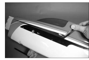
$\Box$  4. Locate the carbon wing tube. Slide the tube into one of the wing panels. It will slide in easily, so do not force it further than it will easily slide.
