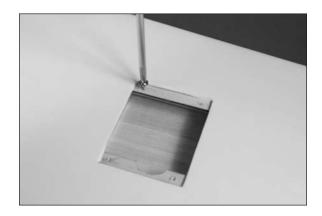
□□ 21. Apply 2–3 drops of thin CA in each hole to harden the surrounding wood. This will help prevent the screws from vibrating loose.
