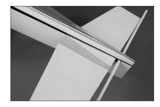
$\Box$  13. Mix 1/2 ounce (15mL) of 15-minute epoxy. Use an epoxy brush to apply the epoxy to the exposed wood on both the top and bottom of the stabilizer. Make sure not to get any epoxy on the elevator.
