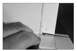
$\Box$  15. Use a #1 Phillips screwdriver to secure the control horn to the elevator using three 2mm x 12mm machine screws and a control horn backplate.
