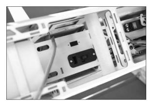
$\Box$  2. Connect the leads from the rudder, elevator and throttle servos to the receiver. Also connect the switch harness and extensions for the ailerons at this time.
