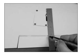
$\square$  2. Center the control horn on the mark made in the previous step. The holes in the control horn will align with the hinge line. Use a felt-tipped pen to mark the locations for the two mounting screws on the aileron.
