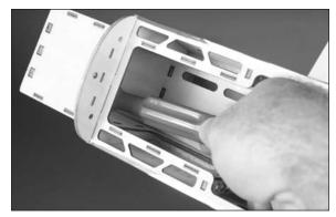
$\Box$  5. Install the blind nuts into the back side of the firewall. Use a 3mm x 20mm socket head bolt and 3mm washer to draw the prongs of the blind nut into the firewall, fully seating them. Use a 2.5mm hex wrench when tightening the socket head bolts.
