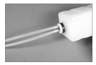
**Important**: We recommend using two colors of tubing on the tank: red on the vent line and the green on the line from the clunk. If a single color is used, make sure to mark them so they can be identified when the tank is inside the fuselage.
