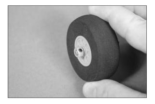
$\square$  8. Insert the wheel assembly into one of the wheel pants. The threaded portion of the axle will fit into the notch of the wheel pant.
