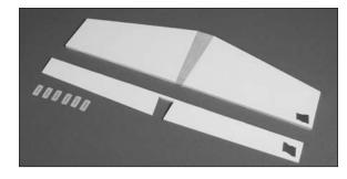
$\Box$  2. Use a pin vise and 1/16-inch (1.5mm) drill bit to drill a hole in the center of each hinge slot. This will provide a tunnel for the CA to wick into, providing a better bond between the wood and hinge when they are glued in position. Prepare both the stabilizer and elevator at this time.
