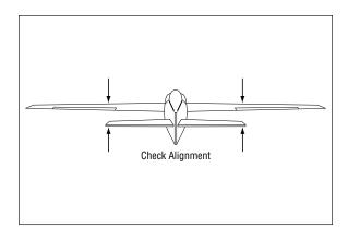
$\Box$  10. Once the alignment has been set, use a felt-tipped pen to mark the outline of the fuselage on the stabilizer. This will allow easy repositioning as it will be removed in the following step.
