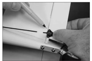
$\Box$  14. Use a pin vise and 5/64-inch (2mm) drill bit to drill the three holes for the control horn mounting screws. Apply 2–3 drops of thin CA in each hole to harden the surrounding wood.
