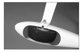
**Note:** Always use threadlock on metal-to-metal fasteners to prevent them from vibrating loose.
