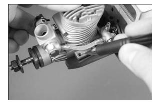
$\Box$  13. Use a drill and 1/8-inch (3mm) drill bit to drill the holes for the engine mounting screws.
