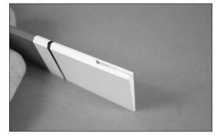
□ 10. Test fit the tail gear wire into the rudder. The wire will rest flush with the hinge line of the rudder as shown. You may need to adjust the groove in the rudder to fit the tail gear wire.
