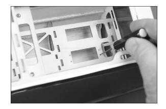
□□ 6. Use a #1 Phillips screwdriver to run a servo mounting screw in each of the holes to cut threads in the surrounding wood. Remove the screw before proceeding to the next step.
