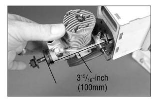
$\Box$  12. Use a pencil to mark the locations for the four engine mounting screws on the engine mount.
