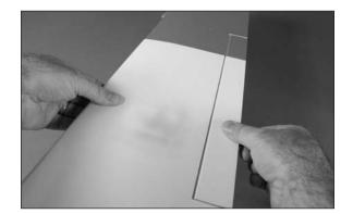
9. Flex the aileron through its range of motion a number of times to break in the hinges. This will reduce the load on the servo for those first flights.
