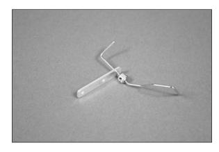
□ 13. Mix a small amount of 15-minute epoxy. Apply the epoxy to the notch in the rudder and the tail gear wire where it fits in the rudder. Insert the wire and use low-tack tape to hold the wire in position until the epoxy cures. Remove any excess epoxy using rubbing alcohol and a paper towel.
