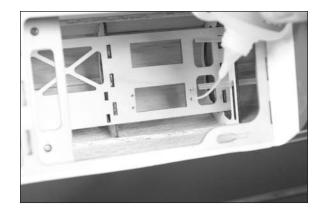
$\square$  8. Secure the elevator servo in the fuselage using the screws provided with the servo and a #1 Phillips screwdriver. Make sure the output of the servo faces to the rear when installed in the fuselage. Route the servo lead through the servo tray in the location shown in the photo.
