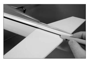
$\Box$  11. Remove the stabilizer from the fuselage. Note the direction of the top and bottom of the stabilizer indicated by the tape placed on it back in step 1. Slide the elevator into the slot, noting the top and bottom to match that of the stabilizer that was just removed.
