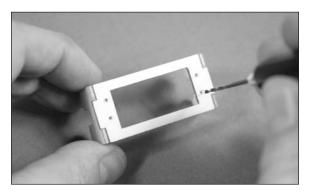
□ 5. Use a #1 Phillips screwdriver to run a servo mounting screw in each of the holes to cut threads in the surrounding wood. Remove the screw before proceeding to the next step.
