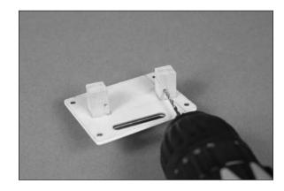
$\Box$  15. Use a #1 Phillips screwdriver to run a servo mounting screw in each of the holes to cut threads in the surrounding wood. Remove the screw before proceeding to the next step.
