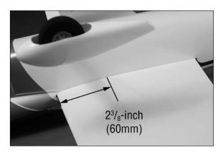
□ 2. When balancing your model, make sure it is assembled and ready for flight. Support the plane upright at the marks made on the wing with your fingers or a commercially available balancing stand. This is the correct balance point for your model.
