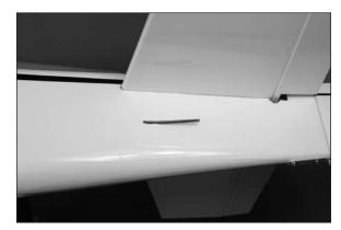
$\Box$  12. Use the radio system to center the elevator servo. Use a #1 Phillips screwdriver and the screw removed from the servo to attach the servo horn to the servo.
