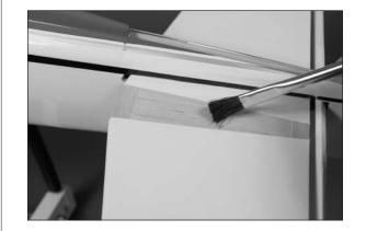
$\Box$  14. Slide the stabilizer in position. Use a paper towel and rubbing alcohol to remove any epoxy that oozes out when the stabilizer is positioned.
