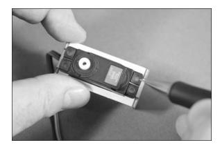
$\Box$  4. Remove the servo from the servo tray. Use a pin vise and 1/16-inch (1.5mm) drill bit to drill the holes for the servo mounting screws.
