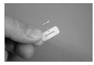
$\Box$  16. Place the hinges in the rudder.
