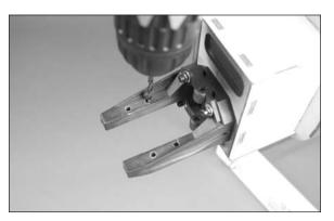
Hint: Use a drill press to drill the holes for the engine mounting bolts so they are nice and straight in the mount.
