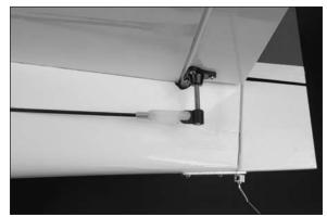
$\Box$  17. Install rudder servo and the 21<sup>7</sup>/<sub>8</sub>-inch (555mm) rudder pushrod following steps 3 through 15. Use the rudder control horn prepared in step 2. The only difference is that the rudder servo mounts on the right-hand side and the pushrod routes out the right side of the fuselage.
