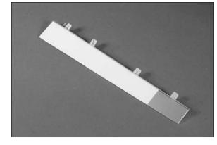
$\Box\Box$  5. Slide the hinges into the slots in the wing panel.
