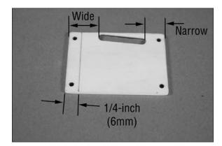
□□ 9. Position the servo on the cover so the horn is centered in the width of the slot. Align the edge of the servo with the line drawn in the previous step. Use a pencil to mark the location of the servo mounting tabs.
