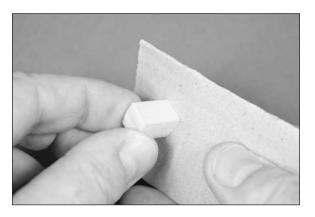
$\Box$  11. Use 5-minute epoxy to glue the square end of the hardwood block to the servo cover using the marks made in step 18. Allow the epoxy to fully cure before proceeding.
