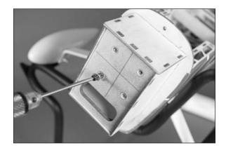
*Hint*: Use a drop of medium CA to attach the blind nut to your finger so it can be installed easily. Make sure it is not glued too well as it may become difficult to break free.
