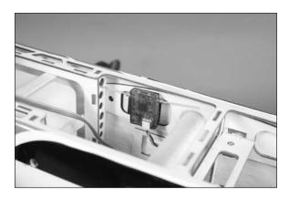
□ 5. Use a hook and loop strap to secure the receiver battery in the fuselage. Make sure to place a piece of foam rudder between the receiver battery and radio tray to isolate the battery from vibrations. Secure the receiver battery lead to the switch harness lead so it does not disconnect accidentally.
