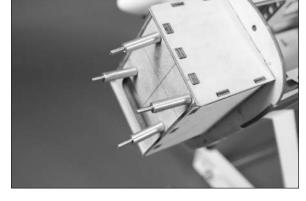
**Note**: The Power 32 will require four  $1^{1}/_{16}$ -inch (27mm) aluminum standoffs. Use four 3/4-inch (22mm) aluminum standoffs for the Power 25 installation.
