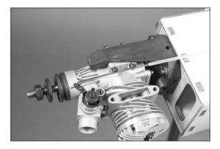
*Hint*: Remove the carburetor to make the installation of the pushrod wire easier.
