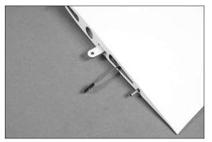
□□ 24. Secure the servo cover and servo to the wing using a #1 Phillips screwdriver and four 2mm x 8mm self-tapping screws.
