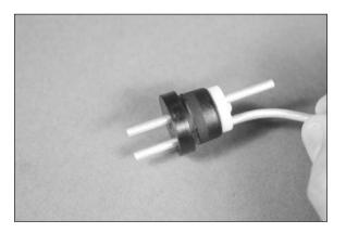
$\Box$  5. Slide the larger stopper plate over the tubing at the front. Start the 3mm x 30mm self-tapping screw using a #1 Phillips screwdriver. The screw only needs to be in far enough to keep the large stopper plate from falling off.
