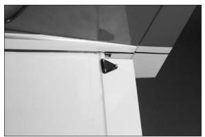
$\Box$  16. With the elevator servo centered, thread the nylon clevis on the pushrod wire. When the clevis is attached, the control surface must be centered as shown.
