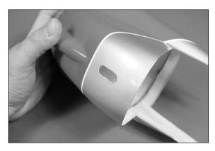
$\Box$  3. To make the installation of the lower cowl mounting screw easier, use a 1/2-inch (13mm) piece of fuel tubing to keep the screw attached to the ball driver as shown.
