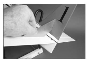
$\Box$  7. Use low-tack tape to hold the fin in position until the epoxy fully cures.
