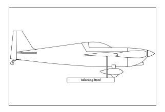
$\Box$  3. You should find the CG to be very close with the components installed as shown in this manual. If the nose of your aircraft hangs low, add weight to the rear of the aircraft. If the tail hangs low, add weight to the nose of the aircraft. Stick-on weights are available at your local hobby store and work well for this purpose.
