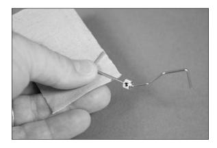
$\Box$  12. Slide the aluminum tail wheel bracket on the tail gear wire. The two larger holes are used for mounting the bracket, while the smaller hole fits over the wire.
