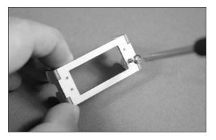
$\Box$  6. Apply 2–3 drops of thin CA in each hole to harden the surrounding wood. This will help prevent the screws from vibrating loose.
