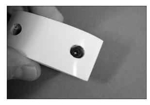
$\Box$  3. Place the landing gear cover assembly on the landing gear. Note that the landing gear will angle forward as shown in the photo. The screws will fit into the mounting holes in the landing gear.
