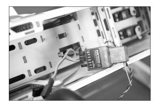
$\Box$  2. Use hook and loop tape to secure the receiver in the fuselage. Make sure to route the leads so they don't interfere with the operation of the servos.
