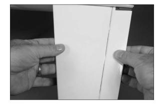
$\Box$  22. Flex the elevator through its range of motion a number of times to break in the hinges. This will reduce the load on the servo for those first flights.
