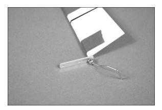
□ 14. Remove the tape from the rudder holding the tail gear wire in position. Use a pin vise and 1/16-inch (1.5mm) drill bit to drill a hole in the center of each hinge slot. This will provide a tunnel for the CA to wick into, providing a better bond between the wood and hinge when they are glued in position. Prepare both the rudder and fin at this time.
