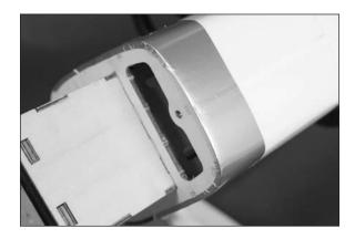
into the fuselage where they can be accessed later. The speed control will attach to the inside of the fuselage, not to the underside of the battery tray.
