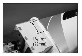
$\Box$  12. Use a pin vise and 7/64-inch (2.5mm) drill bit to drill a hole as close to the engine box as possible for the throttle pushrod tube.
