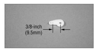
$\Box$  10. Insert the bend on the 20<sup>1</sup>/<sub>4</sub>-inch (514mm) pushrod into the hole enlarged in the previous step. The wire will be on the top of the horn, while the bend will end underneath the horn.
