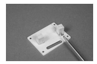
□□ 16. Apply 2–3 drops of thin CA in each hole drilled. Also saturate the front and rear of the block using thin CA to harden the block. This will help keep the block from splitting when the servo mounting screws are installed.
