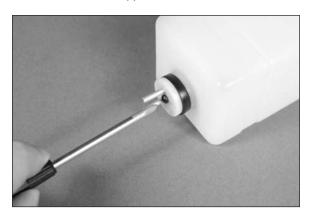
$\Box$  10. Slide the fuel tubing (not included) on the aluminum tubes outside the tank.
