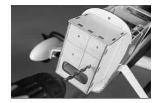
$\Box$  4. Note there is a slight bevel where the blind nut contacts the back side of the firewall. Use a hobby knife or tapered reamer to bevel the inside of the holes to fit the bevel of the blind nut.
