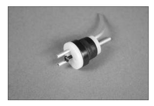
$\Box$  6. Attach the 4<sup>1</sup>/<sub>2</sub>-inch (115mm) piece of fuel tubing to the straight tube. Use a hobby knife to trim the length of the tube to a length of 2<sup>3</sup>/<sub>4</sub>-inch (70mm) as shown in the photo below.
