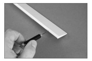
$\square$  3. Place a T-pin in the center of the four hinges removed in step 6. This will center the hinges evenly in the rudder and fin.
