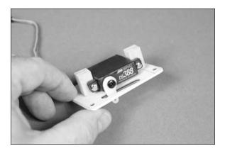
□□ 18. Fit the aileron servo and cover to the wing. Use a pencil to transfer the four positions for the servo cover mounting screws onto the cover rails.
