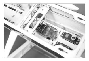
$\Box$  3. Mount the remote receiver in the fuselage away from the main receiver using hook and loop tape. Make sure to orient the antenna on the remote receiver in a different direction than those on the main receiver for the best reception from your radio system.
