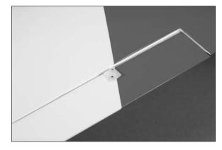
$\Box$  5. Insert the Z-bend of the 2-inch (52mm) linkage in the hole of the servo arm that was enlarged in the previous section of this manual.
