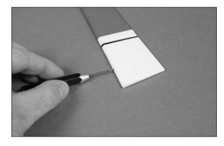
$\Box$  9. Use a hobby knife and #11 blade to cut a groove from the hole drilled in the previous step to the bottom of the rudder for the tail gear wire.
