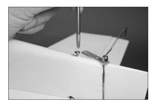
□ 25. Place 2–3 drops of thin CA in each hole to harden the surrounding wood. Doing so will make the screws more secure, preventing them from vibrating loose.
