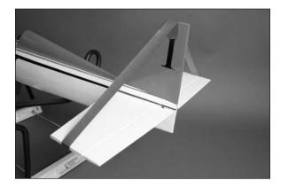
$\square$  8. Use a pin vise and 1/16-inch (1.5mm) drill bit to drill a hole that is 1/2-inch (13mm) deep 7/8-inch (22mm) from the bottom of the rudder.
