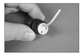
$\Box$  4. Slide the 1<sup>7</sup>/<sub>8</sub>-inch (48mm) aluminum tube through the stopper. Position the front of the tube even with the bent tube as shown.
