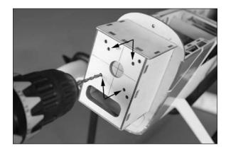
$\Box$  3. Use a drill and 3/16-inch (5mm) drill bit to enlarge the holes in the firewall.
