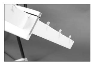
□ 18. Carefully position the elevator so the hinges are inserted into the stabilizer. Make sure that all the hinges get installed, and that none get folded over accidentally. The elevator will fit tightly against the stabilizer as shown. Use the T-pins as handles to help in positioning the hinges.
