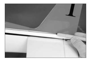
$\Box$  3. Remove the fin from the fuselage. Use a straight edge and hobby knife with a new #11 blade to trim the covering 1/16-inch (1.5mm) below the line on the fin to expose the underlying wood.
