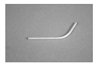
*Hint*: Use a solid round object such as a paint can to bend the tube around to help reduce the chance of kinking the tubing.
