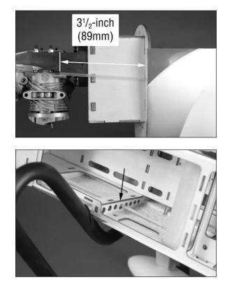
$\Box$  15. Apply 2–3 drops of medium CA where the pushrod tube passes through the formers to secure its location.
