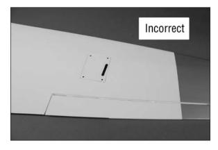
**8**. Use a pencil and ruler to draw a line on the cover 1/4-inch (6mm) from the edge of the cover. The line is located on the end of the cover that has the wider area between the slot and edge of the cover.
