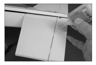
**Note**: Do not use CA accelerator on the hinges. The CA must be allowed time to soak into the hinge and surrounding wood to provide the best bond for the hinge.
