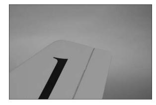
$\Box$  19. Saturate each hinge using thin CA on both the top and bottom of the hinge. Allow the CA to fully cure before proceeding.
