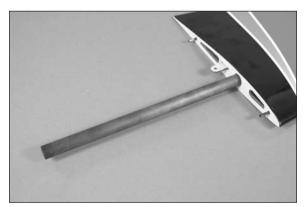
$\Box$  3. Slide the tube and wing panel into position on the fuselage. The wing will fit tight against the fuselage when installed.
