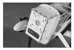
$\Box$  2. Use a drill and 1/8-inch (3mm) drill bit to drill the four holes for mounting the engine. Use the inner set of holes as shown below.
