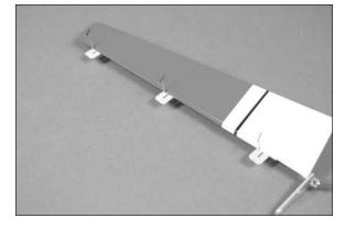
$\Box$  17. Remove the tape placed on the fin and stabilizer in step 7. Slide the hinges into the slots in the rudder.
