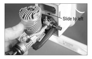
$\Box$  11. Position the engine so the face of the drive washer is  $3^{15/}_{16}$ -inch (100mm) forward of the firewall. Make sure to measure from the firewall where the mount is located, not the edges of the engine box.
