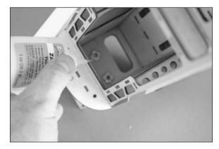
$\Box$  7. Use side cutters to remove the portion of the engine mount as shown in the photo.
