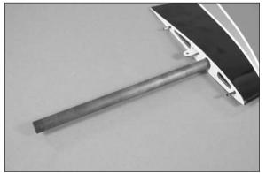
$\Box$  5. Slide the tube and wing panel into position on the fuselage. The wing will fit tight against the fuselage when installed.
