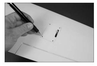
$\Box$  19. Remove the cover and servo from the wing. Use a pin vise and 1/16-inch (1.5mm) drill bit to drill the four holes for the cover mounting screws. Make sure not to accidentally drill through the top of the wing.
