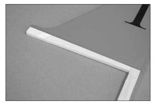
**Note**: When cutting through the covering, use very light pressure or a hot knife to trim the covering. If the underlying wood becomes damaged, the fin may fail in flight, causing the loss of your model.
