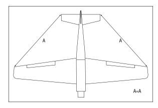
$\Box$  9. Check the alignment of the stabilizer to the wing by standing back 6–8 feet (2–3 meters). The distance between the wing and stabilizer must be equal as shown. If not, lightly sand the opening in the fuselage for the stabilizer to correct the alignment.
