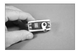
$\Box$  10. Use medium CA to glue the throttle servo tray in the fuselage. Use care not to glue the servo lead in case the servo must be removed later. Note that the output of the servo faces to the rear of the fuselage.
