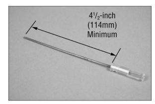
$\Box$  2. (Optional) Use hobby scissors and a rotary tool to make a 3/8-inch x 3/4-inch (9mm x 19mm) slot in the bottom of the cowl to access the lower mounting screw if your ball driver is less than  $4^{1}/_{2}$  inches (114mm) in length.
