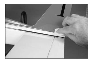
$\Box$  6. Use a square to check that the fin is square to the stabilizer. There will be a slight amount of play to correct for any alignment issues.
