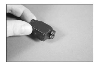
□ 3. Test fit the servo in the throttle servo tray. Use a pencil to transfer the locations of the servo mounting screws on the servo tray.
