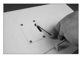
□□ 6. With the radio on and the aileron servo centered, thread the nylon clevis on the pushrod. Thread the clevis on enough so the aileron is centered when the clevis is connected to the outer hole of the control horn shown below.
