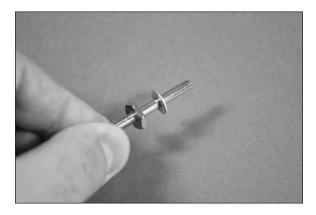
$\Box$  7. Place a drop of light machine oil on the axle so the wheel can rotate easily. Slide the wheel on the axle, then secure it with a 4mm wheel collar. Install the collar so it is flush with the end of the axle. Tighten the setscrew on the flat made in the previous step using a 1.5mm hex wrench.
