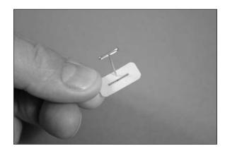
$\Box$  17. Place the hinges in the elevator.
