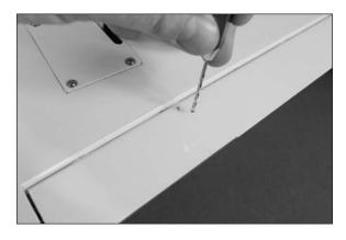
$\Box$  4. Use two 2mm x 12mm machine screws and the control horn backplate to secure the control horn to the aileron. Use a #1 Phillips screwdriver to tighten the screws. Be careful not to crush the underlying wood when installing the control horn.
