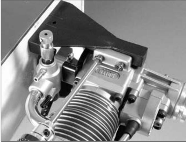
**Cool Tip:** Apply a little bar soap to the threads of the screws to make them easier to thread into the mount. You can also remove the mounts and run the screws through, reattach them to the firewall, and then bolt the engine down.
