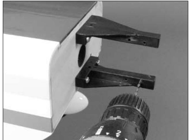
**Cool Tip:** Use a drill press for the best results. This makes holes perfectly perpendicular (square) to the mount.
