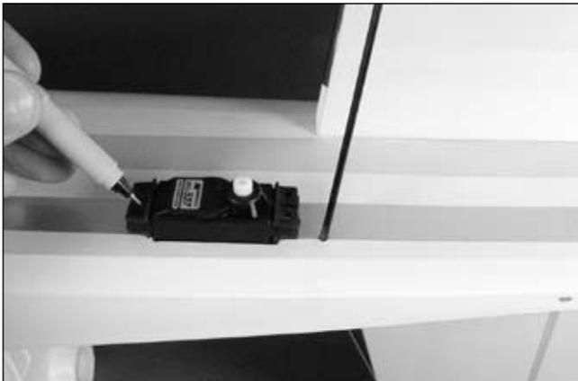
**Cool Tip:** Place a drop of thin CA onto each screw hole to harden the wood around the hole. Allow the CA to fully cure before installing the servos.
