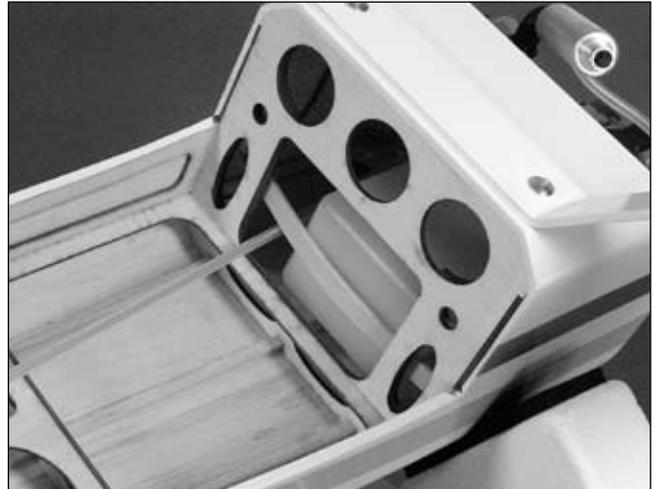
**Cool Tip:** Make sure the rear support brace will not interfere with the installation of the wing.
