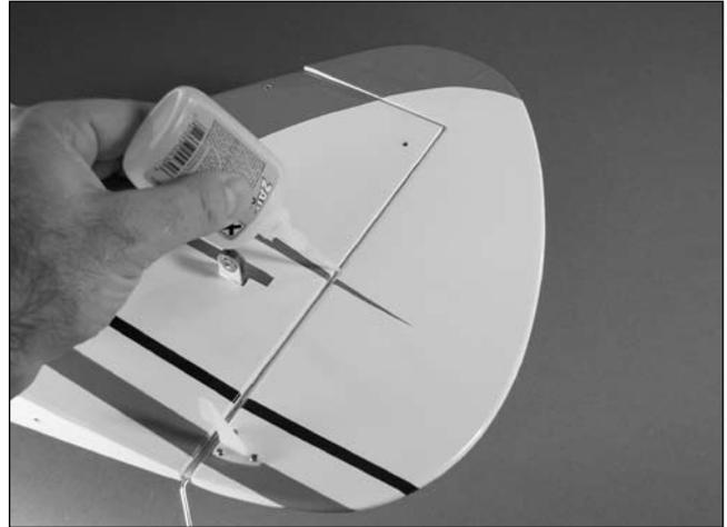
**Note:** The CA must be allowed to cure without the use of accelerator. Using accelerator will not allow the CA to fully soak into the hinge, and could produce a poor bond between the hinges and surrounding wood.
