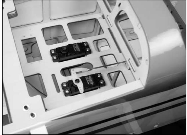
**Note:** The elevator and rudder pushrods are connected to the outer hole on the standard double arm that comes with the servo and they are connected to the middle hole on the control horns for both rudder and elevator.
