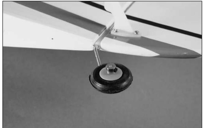
**Note:** Make sure to use threadlock on the setscrews to prevent them from vibrating loose.
