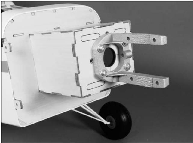
**Note:** Make sure to use threadlock on the screws to prevent them from vibrating loose.
