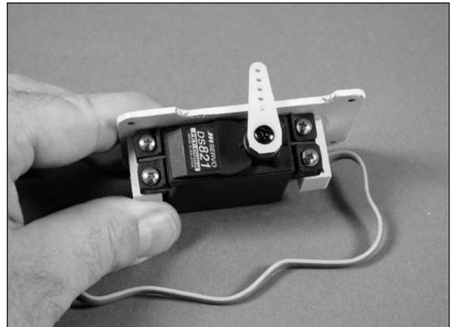
**Note:** When installing the horn on the flap servo, set the throw on the radio to the center position for the flaps.
