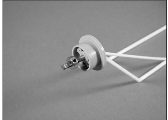
**Note:** Make sure to use threadlock on the setscrews to prevent them from vibrating loose.
