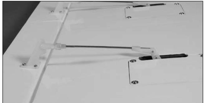
**Note:** When installing the flap linkage, make sure to change the radio to the up flap position before connecting and installing the linkage.
