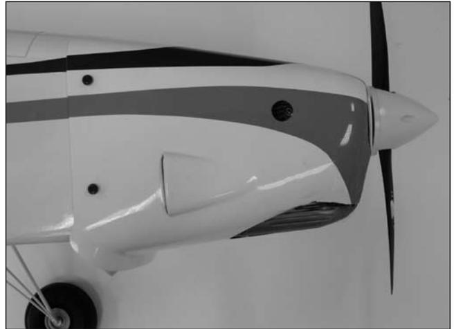
**Note:** We used a Dubro Exhaust Deflector (DUB697) to allow the exhaust to exit the rear opening in the cowl.
