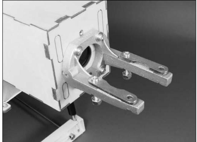
**Note:** The motor mount plates have a textured side that faces the mount when installed.
