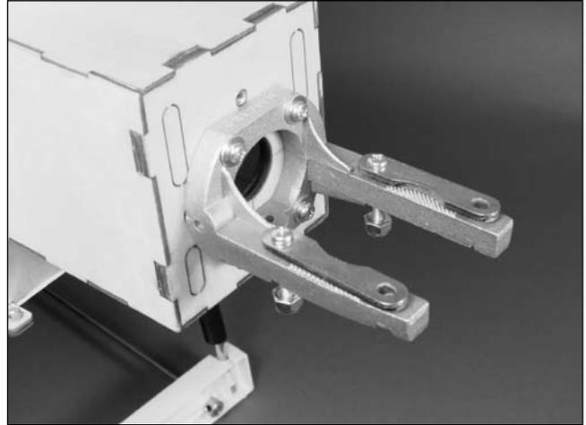
**Note:** The motor mount plates have a textured side that faces the mount when installed.
