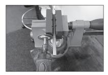
Slide the tubing into the wheel.
