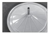
**5.** Check that the tubing is flush with the wheel on both sides before installing the wheel on the axle. Use a flat file to remove any flashing from the tubing or alter its length if needed.
