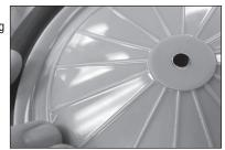
Secure the wheels to the main axle using the wheel collars and M3 x 3 setscrews. The wheel collars are placed on either side of the wheel. Make sure to use a file to make a flat area on the main axle for the setscrews. Apply a drop of threadlock on each setscrew before tightening them using a 1.5mm hex wrench.
