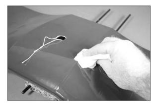
$\Box$  12. Use a covering iron to apply the two strips of covering over the joint between the outer panels and the center panel starting at the trailing edge and wrapping the covering strip around the leading edge in one piece. This will eliminate any seams which could come loose in flight.
