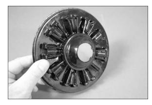
$\Box$  3A. (Glow/Gas Only) Remove the area between the cylinders as shown to clear the carburetor on the engine. Choose the section that has the widest gap between cylinders. This will allow you to see the carburetor to position the dummy engine in the cowl. This hole will be enlarged in the following step.
