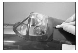
$\Box$  7. Use medium grit sandpaper to lightly sand a 1/4-inch (6mm) wide strip inside the line drawn in the previous step. This will provide a rough surface for the glue to adhere to when gluing the canopy in position.
