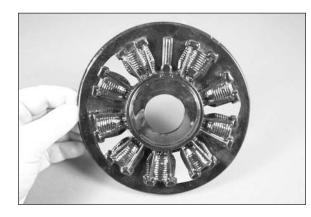
$\Box$  4. Fit the dummy engine over the engine. Trim the dummy engine as necessary so the drive washer is exposed forward of the dummy engine.
