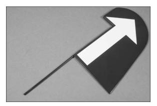
$\Box$  5. Remove the torque rod from the rudder. Use medium grit sandpaper to roughen the torque rod where it will contact the rudder.
