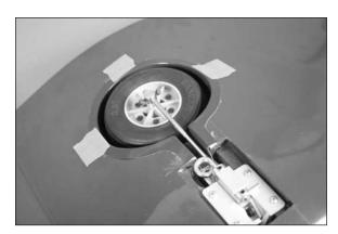
□□ 28. Use the radio to move the gear to the down position. Check that the wheel has a very slight amount of toe-in (front of wheels slightly closer to the wing centerline) in relationship to the wing centerline. This will make takeoff much easier. Cycle the retract a few times and adjust the position of the wheel on the axle and the wheel well if necessary so they do not contact each other while operating the retracts.
