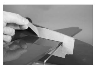
$\Box$  18. Once the epoxy fully cures, the wing can be removed from the fuselage by removing the two 8-32 bolts using a 9/64-inch hex wrench.
