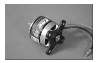
$\Box$  11. Attach the propeller adapter on the motor using the hardware provided with the adapter.
