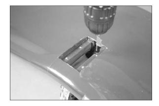
□□ 8. Use a #2 Phillips screwdriver to thread a 3mm x 15mm black counter sunk screw into each of the four holes drilled in the previous step. This will cut threads into the surrounding wood. Remove the screw before proceeding to the next step.
