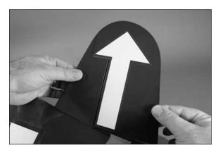
$\Box$  30. Break in the hinges by moving the rudder through its range of throw a number of times.
