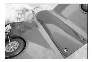
$\Box$  14. Remove the waxed paper from the fuselage to complete the belly pan installation. Leave the wing attached to the fuselage so the stabilizer can be installed.
