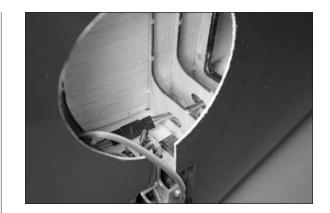
□□ 18. Check the fit of the wheel well into the wing. You may need to use a rotary tool and sanding drum to adjust the opening to allow the well to fit. It may also be necessary to notch the wheel well to clear the top of the retract chassis. Use low-tack tape to hold the wheel well in position. Do not glue the wheel well at this time.
