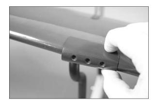
$\Box$  7. Use a drill and 1/4-inch (6mm) drill bit to drill the remaining two locations so the machine gun can rest tightly against the leading edge of the wing.
