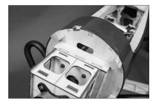
□ 14. Use hook and loop tape to secure the ESC to the bottom of the motor box. Use a tie-wrap to secure the ESC so it won't move from its position. Secure a 6-inch (152mm) servo extension to the receiver lead of the ESC. Pass the leads for the receiver, battery and switch harness though the opening made in the previous step.
