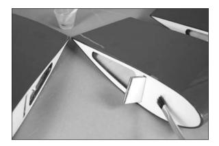
□ 10. Slide the outer and center panels together. Make sure to guide the strings in the wing panels through the hole in the center panel. Wrap a piece of low-tack tape around the leading and trailing edges to keep the panels in alignment. Use a piece of low-tack tape to hold the panels tightly together until the epoxy fully cures.
