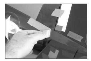
$\Box$  22. Remove the rudder from the fin, leaving the torque rod in the fuselage. Place a T-pin in the center of two hinges. Insert the hinges into the rudder as shown.
