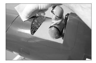
$\Box$  8. Use medium grit sandpaper to lightly sand a 1/4inch (6mm) wide strip inside the canopy. This will provide a rough surface for the glue to adhere to when gluing the canopy in position.
