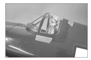
$\Box$  10. Measure back 2<sup>1</sup>/<sub>2</sub>-inches (63mm) and use a hobby knife with a #11 blade to cut a small opening for the antenna mast. Start small and work up until the mast just fits into the opening.
