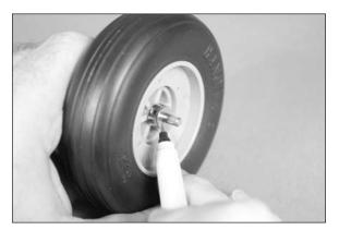
$\Box$  22. Remove the wheel and wheel collar from the axle. Use a rotary tool and cutoff wheel to trim the length of the axle at the mark made in the previous step. Use a flat file to remove any burrs left from trimming the axle.
