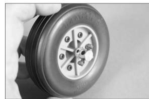
$\Box$  21. Slide the wheel collar from the kit (this collar has a chrome finish) onto the axle. With the axle pressed against the backside of the wheel, use a felt-tipped pen to mark the axle at the edge of the wheel collar.
