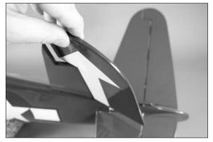
$\Box$  31. With the rudder centered, make sure the balsa fairing is directly under the rudder. Use a felt-tipped pen to trace the outline of the fairing onto the top of the fuselage.
