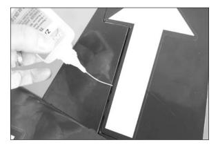
*Important*: Allow the CA to cure WITHOUT using CA accelerator. This is necessary to allow the CA to soak into the hinge, creating the best bond between the hinge and surrounding wood.
