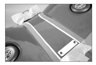
$\Box$  12. Mix 1/2 ounce (15mL) of 30-minute epoxy. Use an epoxy brush to coat the exposed wood on the bottom of the wing. You will want a nice build-up of epoxy to guarantee that it fully contacts the belly pan.
