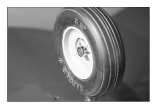
□□ 15. Slide the wheel collar installed in step 10 against the wheel, but not so tight as it prevents the wheel from rotating smoothly. Use a 1.5mm hex wrench (included) to tighten the setscrew. Remember to use threadlock on the setscrew to prevent it from vibrating loose.
