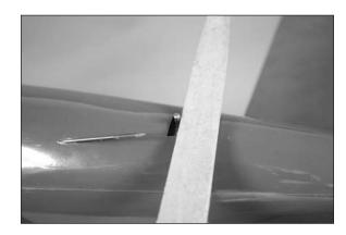
wheel aligned to the fuselage centerline. Tighten the setscrew to mark the location of the setscrew on the tail wheel wire. Remove the wire and use a flat file to file a flat on the tail wheel wire for the setscrew in the adapter.
