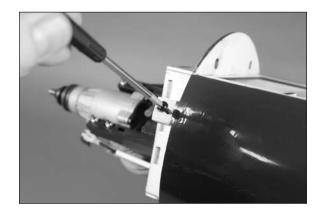
□ 10. Apply 2–3 drops of thin CA in each hole drilled. This will harden the surrounding wood, making the screws more secure when installed.
