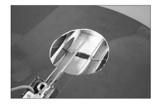
$\Box$  16. Use a hobby knife and #11 blade to remove the rib sections from inside the wing to allow the installation of the wheel well. The ribs have been laser cut to aid in their removal.
