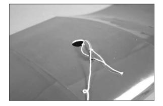
**Note**: Place the drill bit in the drill chuck as far as possible to help prevent accidentally drilling through the top of the wing accidentally.
