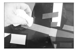
*Important*: If there isn't a fair amount of epoxy to remove, you have not used enough to glue the fin in the fuselage. Remove the fin and apply more epoxy so there is a fair amount of epoxy oozing out when the fin is inserted in the fuselage.
