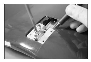
$\Box$  7. Place a 5/64-inch (2mm) drill bit in the drill. Wrap a piece of tape around the drill bit 3/4-inch (19mm) from the end of the drill bit to prevent accidentally drilling through the top of the wing.
