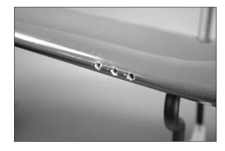
□□ 8. Test fit the machine gun to the wing. You may need to chamfer the holes with a hobby knife and #11 blade slightly to get the machine gun to fit tightly against the wing. Once satisfied with the fit, use canopy glue to secure the machine gun to the wing. Hold the machine gun in position using low-tack tape until the glue cures.
