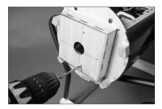
$\Box$  4. Use an 8-32 x 3/4-inch socket head cap screw and #6 washer to draw the four 6-32 blind nuts into the firewall from the inside of the fuselage. Use a 7/64-inch hex wrench to tighten the bolts. Remove the bolt once all the blind nuts are installed.
