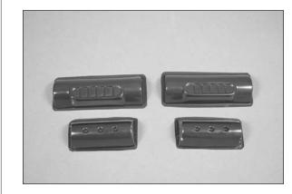
$\Box$  2. Use a hobby knife with a #11 blade and hobby scissors to remove the flashing from the radiator. Also remove the ends so the radiator can fit to the wing.
