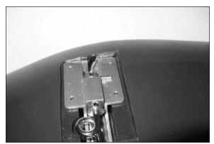
□□ 6. Remove the retract from the wing. Use the radio system to cycle the retract to the down position. Place the retract in the wing. Center the retract frame on the rails, and make sure the retract motor is parallel to the rails. Use a pencil to mark the location for the four mounting screws through the retract frame and onto the rails.
