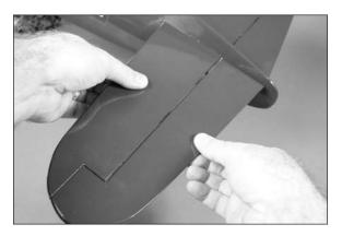
$\Box$  29. Break in the hinges by working the stabilizer up and down a number of times.
