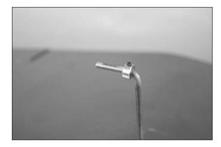
$\Box$  12. Place a drop of light machine oil on the axle.
