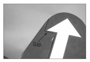
$\Box$  27. Use low-tack tape to tape the balsa fairing in position on the fuselage. Make sure the rudder can move freely and not rub against the fairing before gluing the hinges. The gap in step 26 should match the gap in this step.
