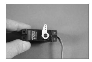
$\Box$  5. Place the servo on the cover, centering the servo horn in the opening. Use a pencil to mark the locations for the servo mounting blocks on the servo cover.
