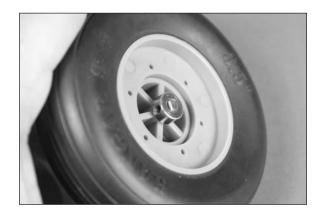
**Note**: If you choose to use a 1.5mm ball driver to tighten the setscrew make a small notch in the wheel hub to reduce the angle of the hex wrench so it fits the setscrew better and to reduce the change of stripping the setscrew.
