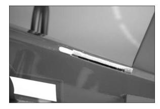
$\Box$  16. Place low-tack tape 1/16-inch (1.5mm) around the outside of the opening in the fuselage for the fin.
