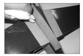
$\Box$  17. After around 25 minutes, before the epoxy fully cures, carefully remove the tape from around the stabilizer. Pull the tape away from the fuselage, being careful not to disturb the position of the stabilizer. This will allow the epoxy to flow out slightly, leaving a fillet between the fuselage and stabilizer. Allow the epoxy to fully cure before disturbing the airframe.
