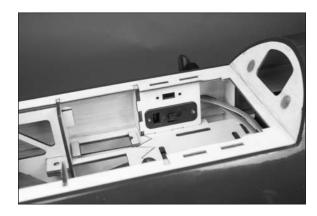
$\Box$  14. Use the hook and loop strap to secure the receiver battery in the fuselage. Make sure to use foam rubber at any point the battery may contact the airframe to protect it from vibrations. Plug the battery into the switch harness at this time as well.
