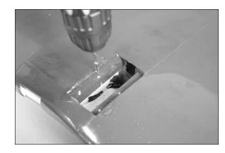
$\Box$  9. Use a #2 Phillips screwdriver to thread a #4 x 3/4inch sheet metal screw into each of the four holes drilled in the previous step, This will cut threads into the surrounding wood. Remove the screw before proceeding to the next step.
