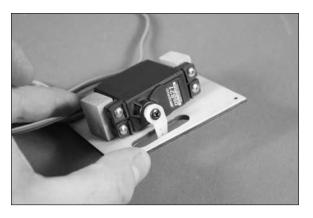
□□ 13. Secure a 12-inch (305mm) servo extension to the aileron servo lead using string or a commercially available connector. Use tape to temporarily attach the extension if you are installing the optional retracts.
