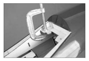
*Hint*: Use a mixing stick between the plate and clamp to protect the plate while tightening the clamp.
