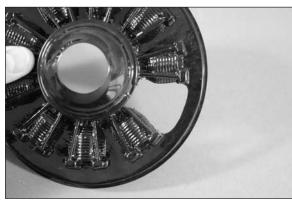
$\Box$  3B. (EP Only) Remove the material between four of the cylinders to allow cooling air to pass over the motor and speed control.
