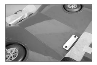
$\Box$  9. Position the fiberglass belly pan on the bottom of the fuselage, aligning it with the contour of the fuselage. Use a felt-tipped pen to trace the outline of the belly pan onto the wing.
