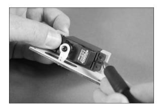
$\Box$  9. Use a drill and 1/16-inch (1.5mm) drill bit to drill the holes for the four mounting screws.
