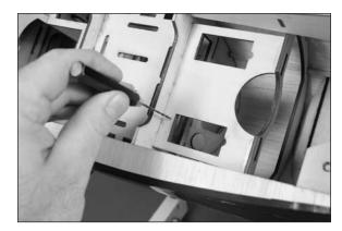
□□ 5. Use a #1 Phillips screwdriver to run a servo mounting screw in each of the four holes. Make sure to remove the screw before proceeding to the next step.
