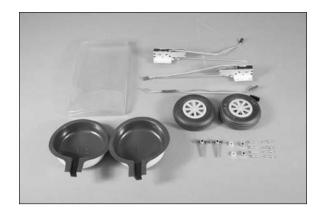
$\Box$  2. Use the radio system to extend the retracts to the open position. Use a rotary tool and cutoff wheel to trim the retract strut length to 4<sup>1</sup>/<sub>8</sub> inches (105mm) from the top of the wheel collar. Use a flat file to remove any burrs after trimming the strut length.
