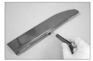
$\Box$  3. Place a T-pin in the center of three hinges. Insert the hinges into the aileron as shown. The hinges have a slot in them and must be installed so the slot is perpendicular to the hinge line of the control surface.
