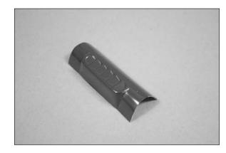
*Hint*: Radius the corners to minimize catching an edge when you wipe the model down with a towel.
