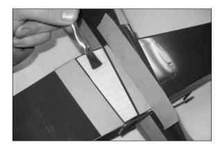
□ 16. Position the stabilizer following steps 5 through 7. Remove any excess epoxy from the stabilizer and fuselage using denatured alcohol and a paper towel.
