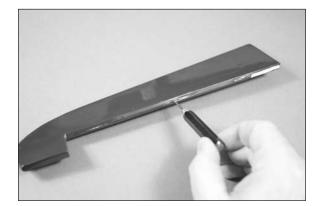
$\Box$  21. Place a T-pin in the center of three hinges. Insert the hinges into the elevator as shown.
