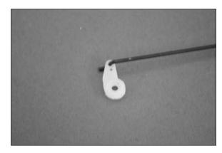
$\Box$  13. (Two-stroke) Center the throttle stick and trim. Slide the pushrod into the tube installed in the fuselage. Attach the servo arm to the throttle servo perpendicular to the throttle centerline. Bend the pushrod slightly so it is parallel to the top of the servo to prevent binding.
