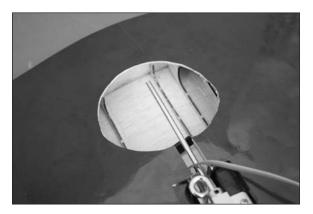
□□ 17. Install the Y-harness included with the retracts and secure it to the lead on the retract using string or dental floss. There are openings in the ribs near the spar to route the aileron and retract servo leads. This will keep the leads from interfering with the fit of the wheel well. Remove the temporary tape from the aileron connection to allow both the retract and aileron extensions to be routed through the wing, as shown in the photo on the following page.
