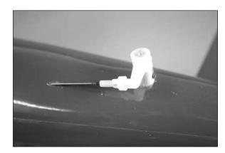
**Note**: The arm on the adapter will angle toward the rear of the fuselage. This is necessary so the pushrod does not bind when operating the rudder.
