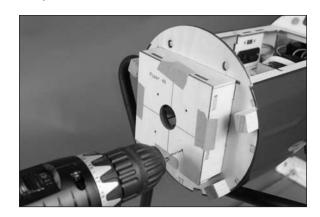
$\Box$  3. Remove the template from the fuselage. Use a drill and 11/64-inch (4.5mm) drill bit to enlarge the holes.
