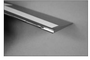
$\Box$  4. Fit the torque rod into the rudder. The front edge of the torque rod will align with the rudder hinge line.
