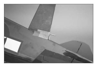
$\Box$  24. Mix a small amount of 30-minute epoxy and apply it to the torque rod and into the hole and slot in the rudder using a toothpick.
