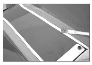
$\Box$  13. Place the belly pan into position on the bottom of the wing. Use low-tack tape to hold the belly pan in position.
