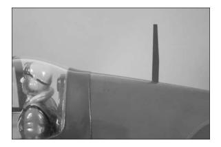
*Hint*: Sight down the top of the fuselage from the front to make sure the antenna mast is vertical and aligned with the fin. There is nothing worse than a crooked mast.
