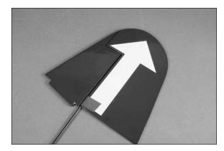
*Hint*: Placing the balance tab against the fin and taping the balsa fairing directly to the bottom of the rudder will produce the same gap for both when the rudder is hinged to the fin later in this section of the manual.
