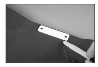
$\Box$  5. Use a hobby knife and a #11 blade to trim the covering 1/16-inch (1.5mm) inside the line drawn on the previous step. Remove the covering from the bottom of the wing.
