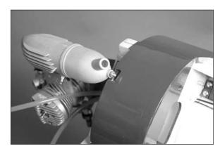
□ 14. (Glow/Gas Only) Connect the fuel lines from the tank to the engine. The line from the vent attaches to the muffler, while the line from the clunk attaches to the carburetor. Fit the cowl over the engine, trimming as necessary to fit over the muffler. Also make an opening for the needle valve so the engine can be tuned without removing the cowl. Make sure to cut the cowl to provide an air outlet for the incoming air that will be cooling the engine.
