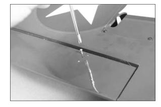
$\Box$  7. Apply 2–3 drops of thin CA in each of the holes that will accept the servo cover mounting screws.
