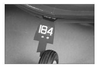
$\Box$  2. When applying the fuel tank decal, we recommend removing as much of the inner clear section of the decal as possible so it can be formed to the curvature of the fuselage. If not trimmed, the decal will wrinkle and not lay flat on the fuselage.
