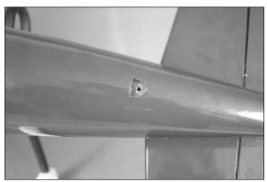
□ 12. Test fit the rudder assembly into the fuselage. Make sure to slide the torque rod into the tube inside the fuselage. Check that the bottom edge of the balsa fairing rests flat on the fuselage. The fin will also rest tightly against the top of the fuselage. If not, remove the covering from the bottom of the fin or even lightly sand the bottom of the fin where it contacts the fuselage to correctly position the balsa fairing.
