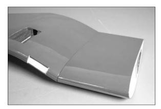
$\Box$  5. Repeat steps 3 and 4 to check the fit of the remaining wing panel to the center panel.
