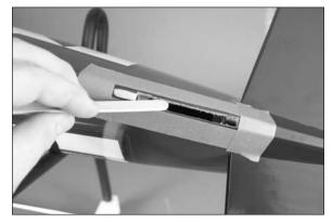
$\Box$  19. Slide the fin into position. Use a paper towel and rubbing alcohol to remove any excess epoxy from the fuselage.
