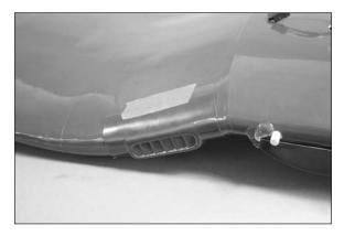
$\Box$  4. Use a hobby knife with a #11 blade and hobby scissors to remove the flashing from the machine gun. Also remove the ends so the machine can fit to the wing.
