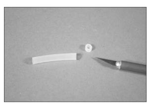
□□ 11. Slide the safety tubing on the nylon clevis. Turn on the radio system and center the aileron stick and trim. This will center the aileron servo. Thread the nylon clevis on the pushrod. Thread the clevis on enough so the aileron is centered when the clevis is connected to the center hole of the control horn shown below. Once set, slide the safety tubing over the forks of the clevis to keep the clevis from opening accidentally.
