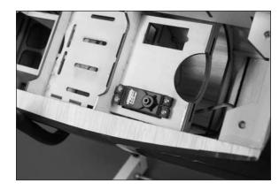
$\Box$  8. Use a pin vise and 5/64-inch (2mm) drill bit to enlarge the hole in the servo arm that is 1/2-inch (13mm) from the center of the arm. Use side cutters to remove any unused arms so they don't interfere with the operation of the servo.
