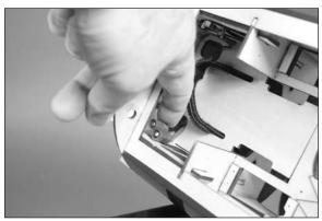
$\Box$  17. The battery is secured in the fuselage using the hook and loop strap. We also recommend using a piece of hook and loop tape between the battery and battery tray to keep the battery from accidentally moving inside the fuselage.
