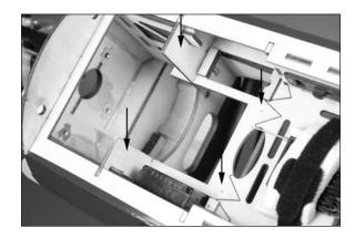
$\Box$  18. Inspect the fuel tank to determine the location of the lines that will connect to the muffler and carburetor. Also note the orientation of the vent line inside the tank.
