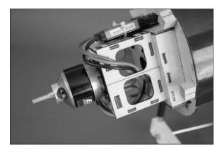
**Note**: If you are installing an E-flite motor and speed control, you can match the colors from the motor and ESC. This will result in the motor rotating the correct direction for your model.
