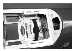
□ 17. Mount the remote receiver in the airframe using hook and loop tape. Make sure the antenna on the remote receiver are 90-degrees in relationship to the main receiver antenna. Place the remote receiver as far away from the main receiver as possible for the best radio reception.
