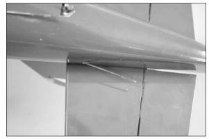
$\Box$  12. Slide the hatch forward then lift it up at the rear. There are tabs near the rear edge that must clear the top of the fuselage before lifting the hatch, so make sure the hatch is slid forward as far as possible before removal.
