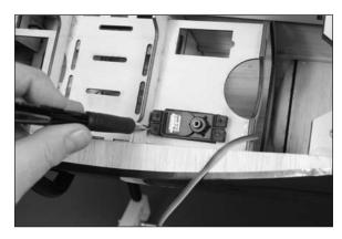
$\Box$  4. Use a pin vise and 1/16-inch (1.5mm) drill bit to drill the holes for the four mounting screws.
