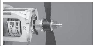
□ 5. Temporarily mount the prop adapter and the propeller to the motor shaft. Use an 8mm wrench to tighten the prop nut while holding the collet with a 10mm wrench to lock the prop adapter onto the shaft.
