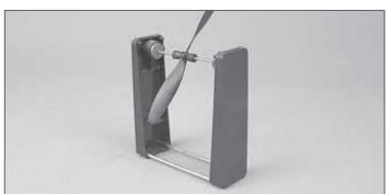
1. For optimum performance and motor efficiency balance the propeller using a Top Flite® Precision Magnetic Prop Balancer (TOPQ5700) or other suitable balancer. Use a hobby knife or sandpaper to sand the one side of the heavier blade until you can get the prop to balance.
