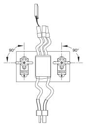
□ 2. With the transmitter on, the trims centered and the motor battery connected to the receiver, fit the servo arms on the rudder and elevator servos so the arms will be 90-degrees (or as close as 90-degrees as possible) to the servos.
