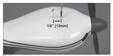
☐ 11. Drill a 1/16" [1.6mm] hole trough the cowl and the cowl mounting block 1/2" [13mm] ahead of the pin in the top of the motor pod—this should put the screw hole right in the middle of the cowl mounting block. Screw in one of the three larger wood screws that came with this kit.
