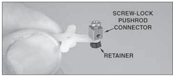
☐ 3. If necessary, use a hobby knife to carefully enlarge the hole in the elevator servo arm. Then connect a small, brass
