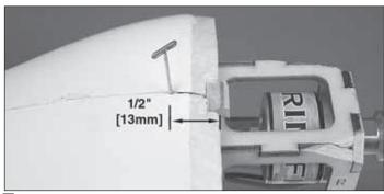
☐ 7. Insert a pin into the motor pod 1/2" [13mm] behind the middle of the wood block for the top cowl mounting screw.
