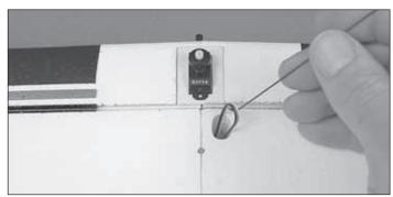
☐ 1. Use a brass tube sharpened on the end or a hobby knife to cut a hole in the bottom of the wing where shown for the aileron servo wire. Use one of the aileron pushrod wires with the 90° bend on the end to pull the servo wire up through.
