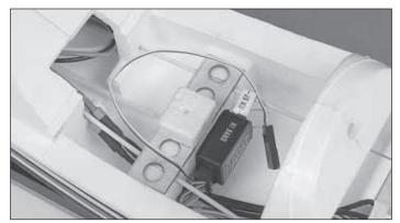
☐ 13. Use the included Velcro hook-and-loop material (or optional double-sided foam mounting tape—not included) to mount the receiver where desired. The location shown is preferable because all the wires can easily reach and the receiver will be raised off the cabin floor, making it less likely to get wet if any water leaks in.
