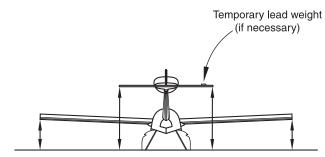
☐ 1. Temporarily mount the wing to the fuselage. With the plane resting in its building cradle, measure the distance from the bottom of both wing tips down to your workbench. Adjust the plane in the cradle until both distances are equal.
