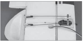
□ 2. The same as you mounted the rudder and elevator servos in the fuse, mount the aileron servo in the wing–only this time use a drill **no larger** than a #58 (.042") [1.07mm] for the servo screw mounting holes. If you don't have the right drill you could use the tip of a #11 blade to make the holes instead. If you do accidentally oversize the holes, they may be filled with medium CA and redrilled.
