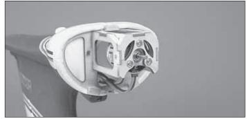
☐ 4. Connect the wires on the motor to the wires in the fuse. Mount the motor with the three 3mm x 6mm Phillips screws that came with this kit and a drop of threadlocker on the threads.
