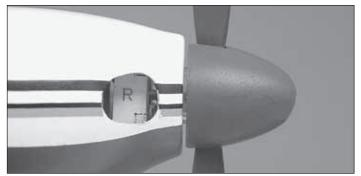
☐ 10. Fit one of the spinners all the way onto the propeller and collet assembly. Adjust the cowl so there will be an approximately 1/16" [1.5mm] gap between the spinner and the cowl.
