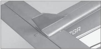
☐ 7. Glue in the fin with the same glue used for the stab—do not clog the receiver antenna tube that comes out of the fuselage by the left side of the fin. View the fin from behind the model to make sure it is vertical.
