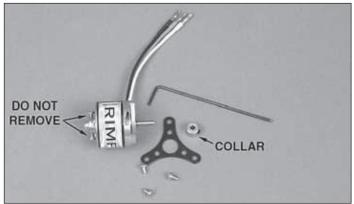
3. Use a 1.5mm Allen wrench to loosen the set screw in the collar on the front of the motor (not included) and remove the collar. Also remove the mounting plate, but leave the prop saver screws in place because they hold in the drive shaft.
