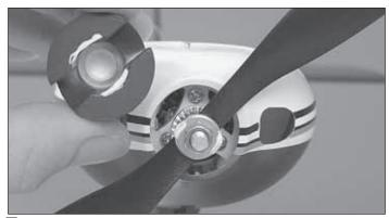
2. Mount the propeller with the included aluminum propeller washer. Use a few dabs of RTV silicone, R/C 56 or waterproof white glue to glue on the spinner. Using just a few dabs of any of the soft glues recommended should allow the spinner to be removed if ever necessary in the future. If the spinner becomes damaged two spares are provided.
