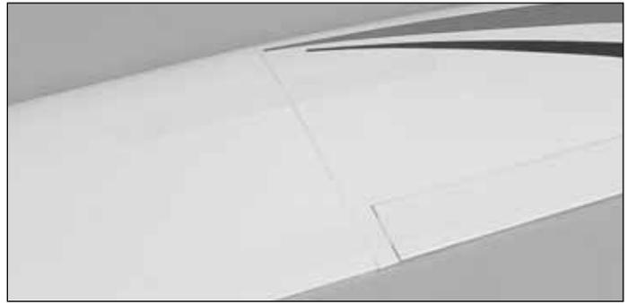
3. Cut away the covering from the servo bay. Using 30-minute epoxy, coat the wing joiner, wing center-section rib, and wing outer panel. Attach the wing outer panel. Route the servo extension from the center-section into the servo bay. Clean up any excess epoxy with denatured alcohol and a paper towel. Align the trailing edge of the center-section and the outer panel. Hold the two in place using masking tape while the epoxy hardens.
