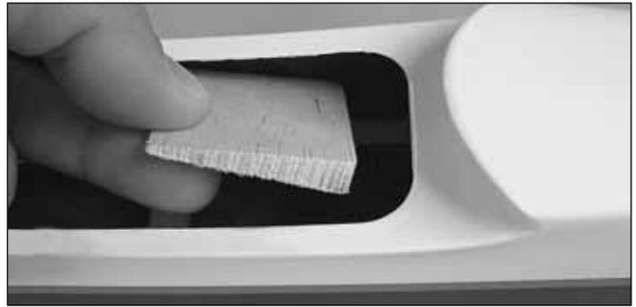
❑ 4. If the battery does not slide forward far enough to fit inside the fuselage, tack glue the hardwood wedge on the battery tray against the forward former. This wedge will lift the front of the battery and it will help it slide through the forward former easily.
