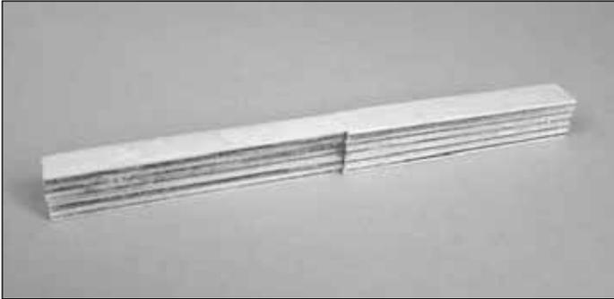
1. Locate five 1/16" [1.6mm] ply wing joiner plates. Mix a generous amount of 6-minute epoxy and glue the plates together. Clean up excess epoxy with denatured alcohol and a paper towel. Allow the epoxy to harden before proceeding.
