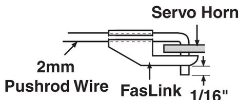
6. Mark the pushrod where it crosses the servo arm. Make a 90° bend at the mark and push through the servo arm. Attach a nylon FasLink and trim off the excess pushrod, leaving approximately 1/16" [1.6mm] past the FasLink. Remove the elevator servo.
