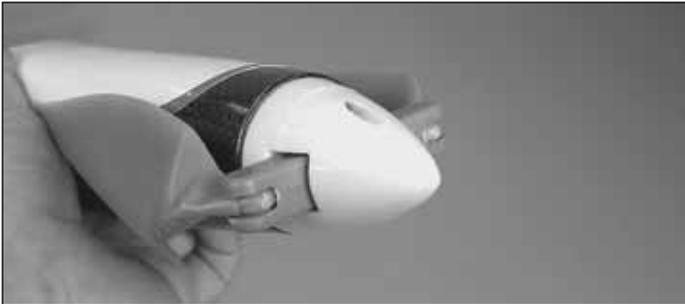
❑ 3. Check for proper motor rotation. Attach the prop adapter, adapter washer, prop, and spinner to the motor shaft as determined by the motor manufacturer.
