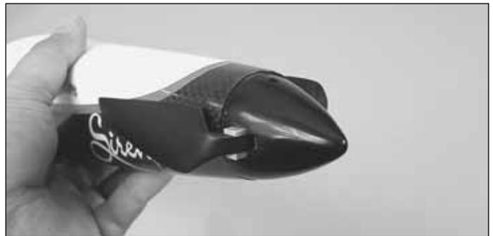
❑ 3. Check for proper motor rotation. Attach the prop adapter, prop, and spinner to the motor shaft as determined by your manufacturer.
