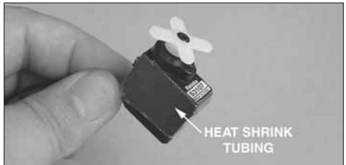
1. Using a piece of Trinity Single Cell heat shrink tubing, fit the tubing over the servo and heat shrink it. This will allow you to easily replace the servo later since the tubing will be glued in place, not the servo.
