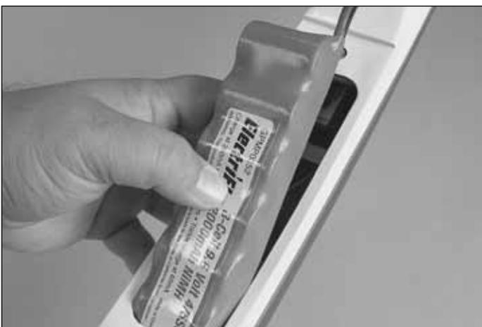
❑ 3. Slide the battery into the radio compartment. **DO NOT CONNECT THE BATTERY TO THE ESC AT THIS TIME.** Use 1/4" [6mm] foam to hold the battery in place. Adding foam to the front or back of the battery compartment can be helpful in shifting the battery location for balancing. The battery will be a tight fit. Glue Velcro with CA or epoxy to the bottom side of the battery and to the battery tray to hold the battery in place.
