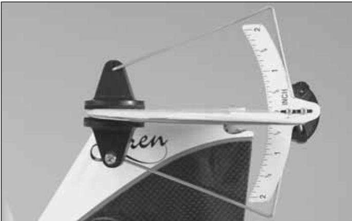
Use a Great Planes AccuThrow™ (or a ruler) to accurately measure and set the control throw of each control surface as indicated in the chart that follows. If your radio does not have dual rates, we recommend setting the throws at the **middle of both rate settings**.
