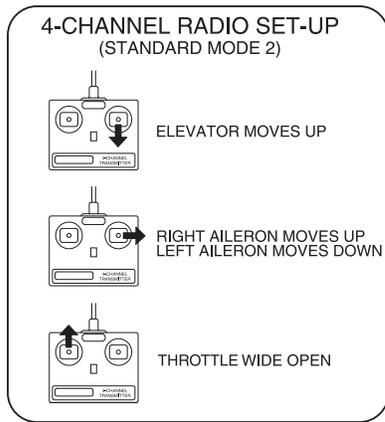
3. Make certain that the control surfaces and the throttle respond in the correct direction as shown in the diagram. If any of the controls respond in the wrong direction, use the servo reversing in the transmitter to reverse the servos connected to those controls. Be certain the control surfaces have remained centered. Adjust if necessary.
