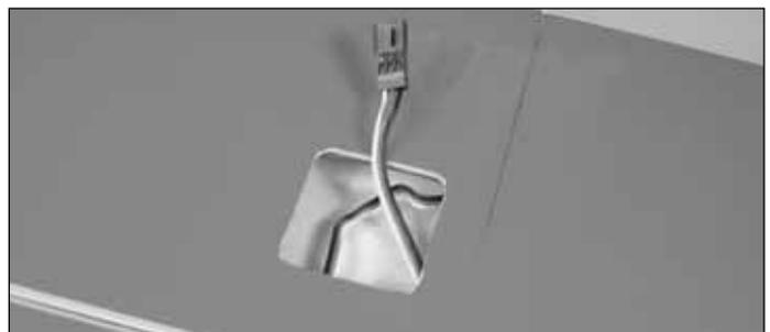
2. Connect the servo lead to the 24" [610mm] servo extension. Secure the connection with a 1-1/2" [38mm] piece of
