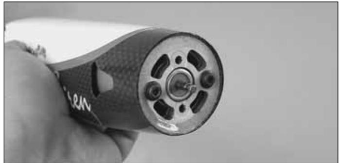
❑ 2. Guide the motor into the nose of the airframe from the inside of the fuselage. Mount the motor to the firewall using the screws that came with the motor and Threadlocker.
