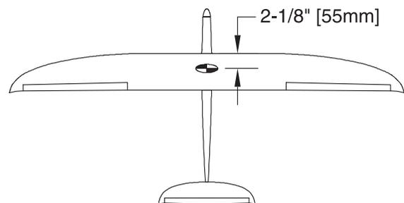
2. With the wing attached to the fuselage and all parts of the model installed (ready to fly), place the model on a Great Planes CG Machine™, or lift it at the balance point you marked.
