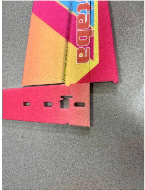
Join the wing and the horizontal fuse and allow to dry.
