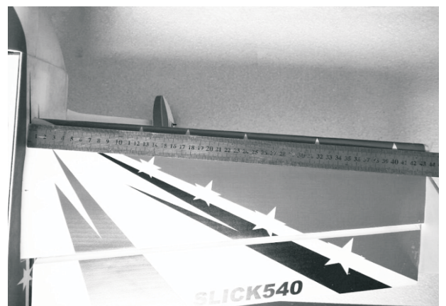
6 .Slowly and carefully insert the wings into the fuselage,so that it is in the center of the wings, using a ruler to measure the same distance between the side
