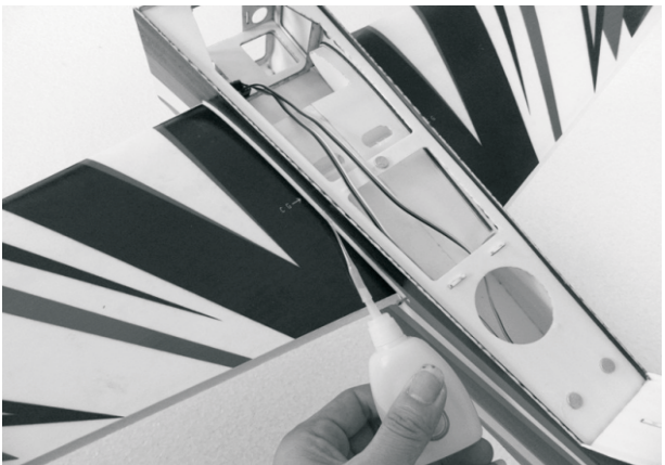
11 . Ensure that the Angle between the wing and both sides of the fuselage is symmetrical, and the contact position between the wing and the fuselage is properly cemented with quick-drying glue (note: do not use too much quick-drying glue, it will corroded the foam inside).
