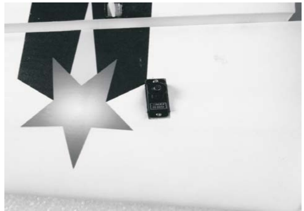
22. Install the aileron servo and secure hinge positions with quick-drying glue. (It is best to leave 1 mm space between ailerons and wings, so that ailerons can swing up and down flexibly)
