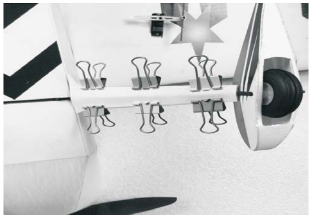
36.To install the landing gear trim, apply foam glue around it and clamp until the glue is completely dry before releasing the clamp.
