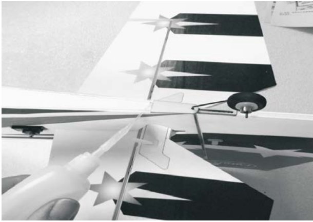
19. Use quick-drying glue to fix the tail wheel bracket to secure the wood pieces.
