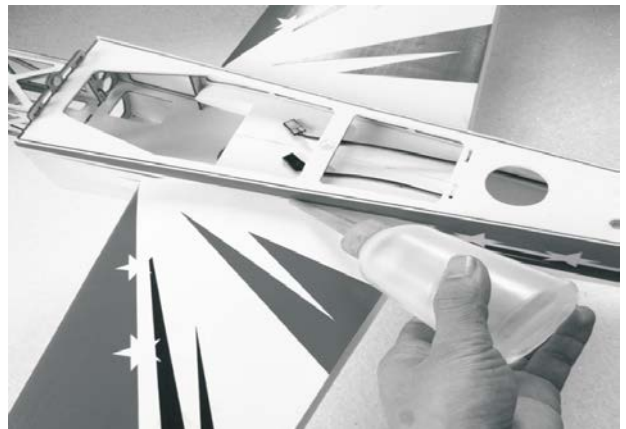
12 . Then use foam glue to reinforce the contact between the wings and the fuselage
