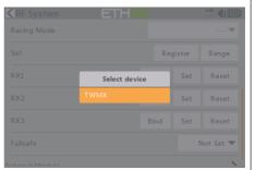
Click the RX to complete the binding after the receiver window pops up, the system will confirm "Bind succeed".
