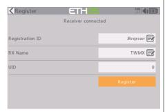
When the "RX Connected" page pops up, press the [REGISTER] to complete the Registration procedure and then power the receiver off.
