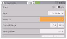
The system assigns the receiver a number for the receiver (Model ID) automatically while creating a new model. (The Model ID can be set from 00 to 63, with the default ID being 1.)
