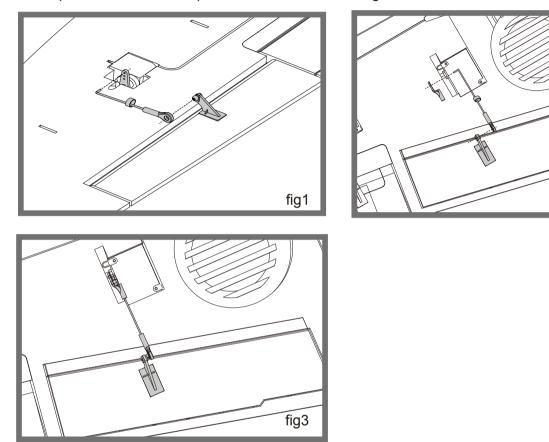
2. Slide the wing tube into the wing holes. Ensure the the connector wires pass through the hole to the top side of the wing. Secure the wing together by installing two brackets where the two wing halves join as shown. Assemble the oil tank using the screw PA2.6\*15mm as shown in Figure6.
