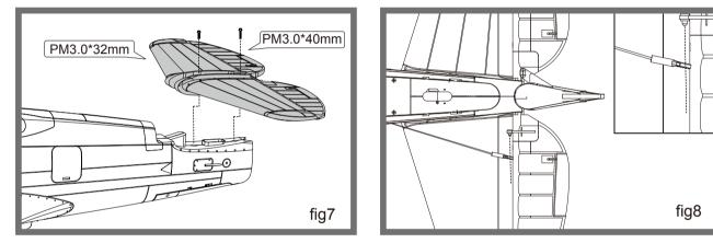
4. Turn over the fuselage so the bottom faces up and feed the connector wires thorough the hole in the fuselage. Secure the wing in place using 4 wing screws.
