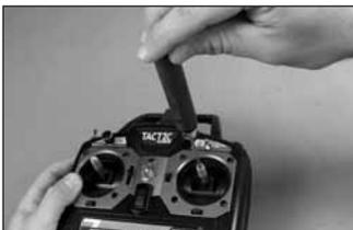
The length of both gimbal sticks can be adjusted as desired. Loosen the set screw inside the center of the stick with a 2mm hex wrench. Rotate the stick end counter-clockwise to lengthen the stick, or clockwise to shorten the stick. Once the desired stick length is found, tighten the set screw with the hex wrench.
