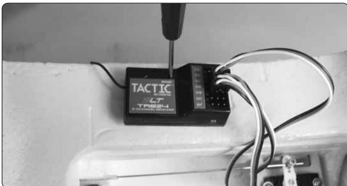
❑ 6. To bind the receiver to the transmitter, remove the receiver from the plane. Make sure the throttle stick is down in the idle
