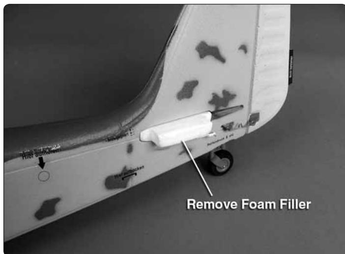
1. Remove the foam filler piece from the horizontal stabilizer opening.
