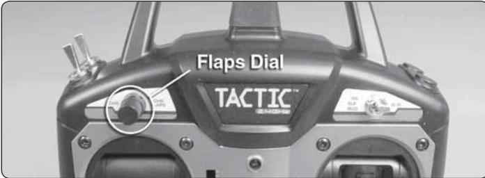
❑ 8 . Operate the flaps from the transmitter. On the Tactic TTX600 the flaps are operated using the dial. Check that the flaps move down the same amount and do not bind in the up position. If one of the flaps moves down more than the other or binds in the up position, loosen the screw in the screw lock pushrod connector and adjust the pushrod until the flaps operate correctly. Check that all the screws in the screw lock pushrod connectors are tight against the pushrods.
