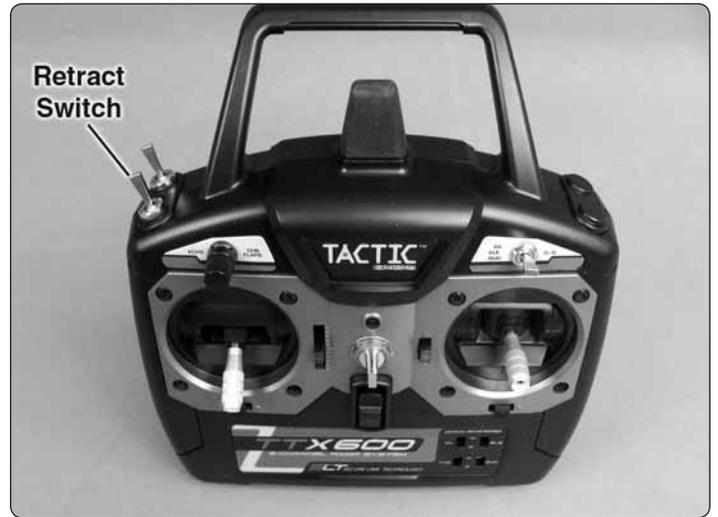
❑ 6. Operate the retracts from the transmitter. On the Tactic TTX600 the retracts are operated from the forward switch. Check that the retracts lock in the down position and do not bind in the up position. If one of the retracts does not lock down or binds when retracted, loosen the screw in the screw lock pushrod connector and adjust the pushrod until the retract operates correctly. Check that all the screws in the screw lock pushrod connectors are tight against the pushrods.
