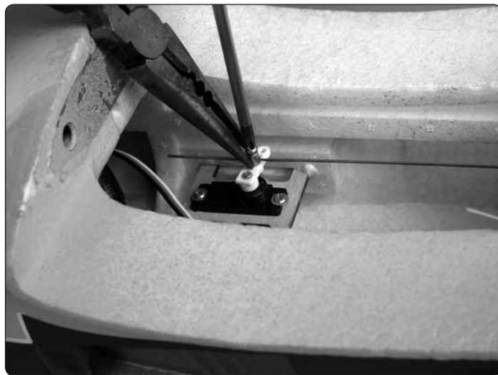
❑ 1. Remove the 2.5 × 5 mm machine screw in the screw lock connector on the elevator servo. Center the elevator and apply a small drop of threadlocker to the threads of the screw. Hold the screw lock connector with a needle nose pliers and reinstall the screw in the screw lock connector, tightening it against the elevator pushrod. Move the elevator stick, checking that the elevator moves in the correct direction.
