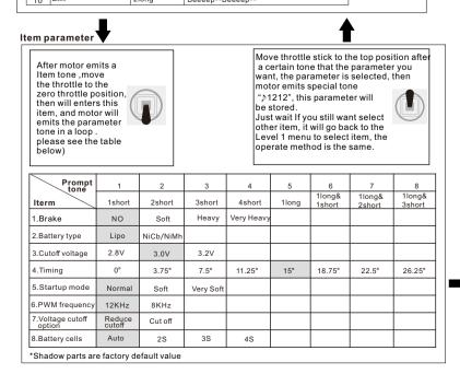
If don't want select other parameter, move throttle to the zero position in 3 seconds, then moto emits special tone "♪765765", it will exit the programm node
