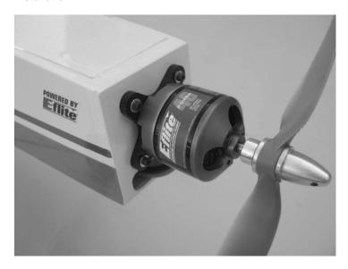
**NOTE:** Photo shows typical installation of motor and x-mount directly to the outside of the firewall. There are other options available including mounting the motor inside the fuselage (requires reversing the shaft direction) or extending the motor further forward using aftermarket mount extensions when using cowls.
