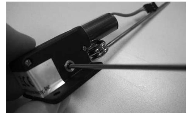
2. Test fit the retract unit in the wing or fuselage to determine the strut length and axle location. Cut the strut to length using a cutoff wheel in a rotary tool.
