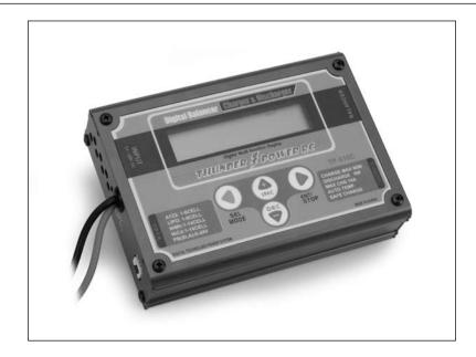
The Thunder Power charger is a charger than can charge any battery currently in use the RC industry. It has software for charging Ni-cd, NiMh, Li-Ion, Li-Po, and A123 cells. Ask for part number #THP610 at your local hobby dealer.
