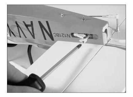
• 8. Screw the nylon control horn in 1/4-inch (6mm). Connect the clevis from the rudder pushrod to the rudder control horn.
