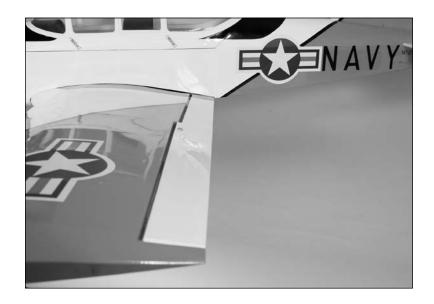
• 12. Check the movement of the aileron using the transmitter. When the elevator/aileron stick is moved right, the right aileron will move up and the left aileron will move down.
