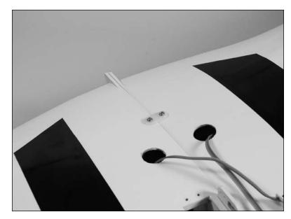
• 7. Slide the lead from the wing panel through the connector stay as shown. The stay will prevent the lead from being unplugged accidentally.
