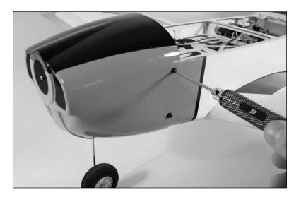
• 4. Use the same 2.5mm hex wrench to check the four screws that secure the motor to the firewall. Once the motor screws are tight, reverse the previous steps to install the cowling, propeller and spinner.
