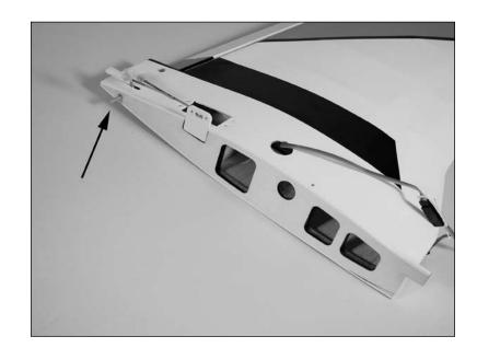
• 4. Slide the wing tube into the wing panel at this time.
