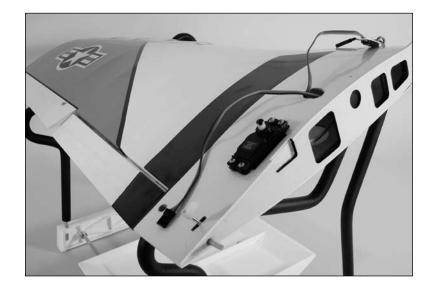
• 6. Use the radio system to center the flap servo. Install the servo arm so it is perpendicular to the servo. You will want equal throw in both directions from this position to operate the flaps.
