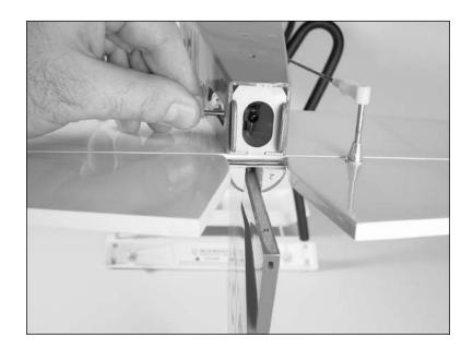
• 4. Slide the fin fully into position. Use two 3mm washers and two 3mm locknuts to secure the fin. Tighten these nuts down using an adjustable wrench.
