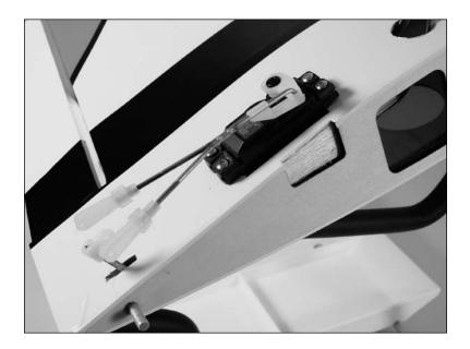
• 10. Use the radio to move the flap servo to the "UP" position. The servo arm will face toward the leading edge of the wing. Connect the clevis to the flap control horn. Check that the flap is aligned with the wing. If not, thread the clevis in or out until the flap is aligned with the wing.
