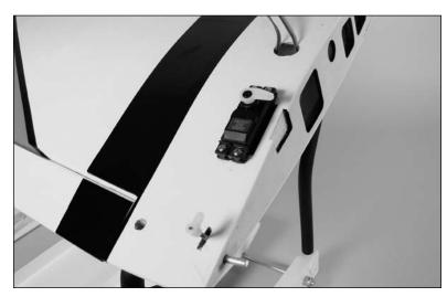
• 7. Use a pin drill and 5/64-inch (2mm) drill bit to enlarge the outer hole of the servo arm.
