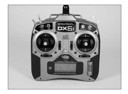
3. Plug the motor battery into the speed control. Set the throttle stick to low throttle and turn on the speed control. You will hear a series of beeps or tones when you plug the battery in. During this process it is normal for the prop to pulse slightly as the ESC powers up. Please ensure you are not in line with the prop or in front of it during power up.
