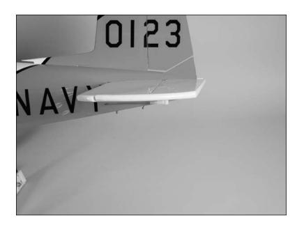
• 6. Check the movement of the elevator with the radio system. Pulling the elevator/aileron stick (right stick on the transmitter) back will make the airplane elevator move up.
