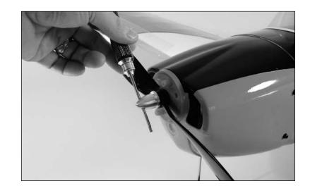
• 3. To check that the motor is secure to the firewall, you will first need to remove the spinner. Use a 2.5mm hex wrench to remove the four screws that secure the cowling to the fuselage.
