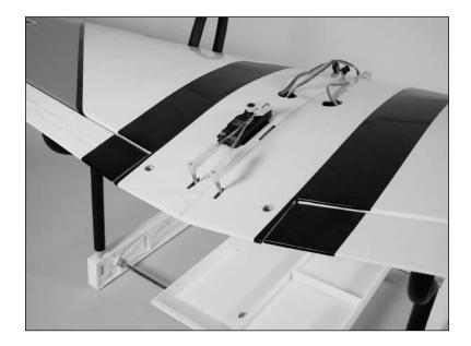
• 12. Use the radio system to set the position for the flap. It may be necessary to use the radio system to change the amount of throw electronically to match those in the following images. Your goal here is to mimic the flap settings from the previous section.
