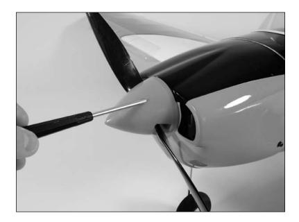
• 2. Check that the propeller adapter is tight using a hex wrench or screwdriver that fits into the hole in the adapter. You will turn this nut counterclockwise to loosen or clockwise to tighten.
