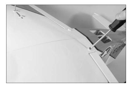
5. Plug the aileron lead into the receiver in the slot marked *AILE*. (The flap servo is plugged into the AUX1 slot of the receiver when the optional flaps have been installed.) Replace the canopy back onto the fuselage. You will want to make sure you have the wires pressed down flat and to the side of the receiver before installing the top hatch.
