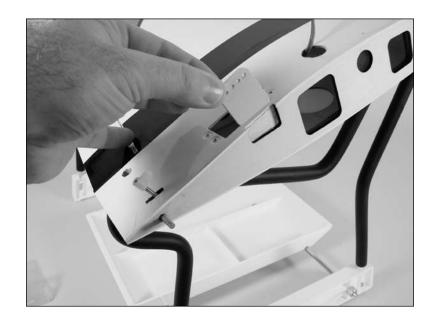
• 2. Position the flap servo in the wing. Use a felt-tipped pen to mark the locations for the four servo mounting screws.
