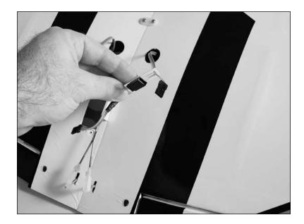
• 8. Rotate the lead in the stay so the colors align with those of the lead already installed. Plug the two connectors together and slide them tight against the stay.
