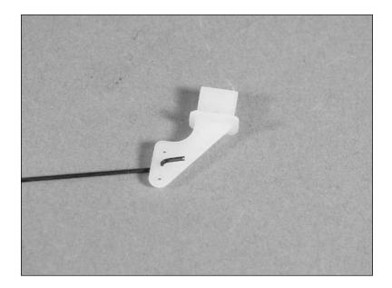
• • • • 2. Slide the pushrod wire into the pre-installed pushrod tube in the fuselage.
