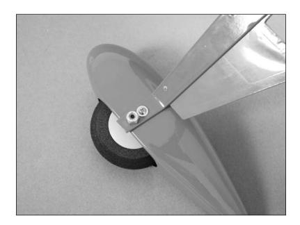
• 5. Repeat Steps 6 through 9 to install the remaining wheel pant.
