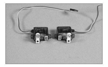
○ ○ 6. Secure a 6-inch (152mm) servo extension to the servo lead using your favorite brand of servo wire keeper or tape.
