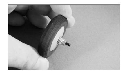
○ ○ 4. Pass the screw into the lower hole in the landing gear. Secure the wheel using a 4-40 locknut.
