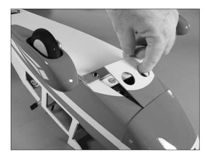
• 4. Install the battery in the fuselage using the 8-inch (204mm) hook and loop strap. Replace the battery door once the battery has been installed.
