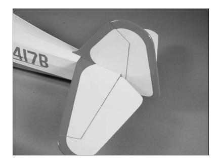
• 4. Trace the outline of the fuselage on the bottom of the stabilizer using a felt-tipped pen.
