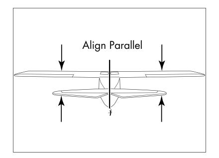
• 9. Apply 30-minute epoxy to the exposed wood of the stabilizer and to the fuselage where the stabilizer will rest. Place the tail assembly on the fuselage and double-check all alignments made. Allow the epoxy to fully cure before moving your airframe.
