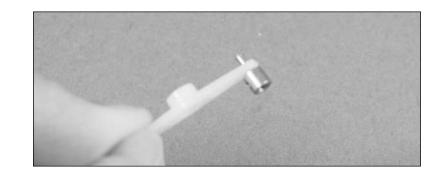
○ ○ 3. Use a pushrod connector backplate to secure the connector to the servo arm.
