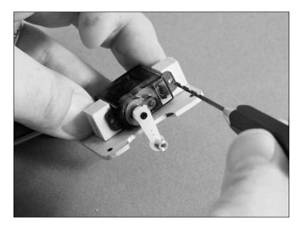
••• 12. Use the hardware provided with the servo to secure it to the blocks using a #1 Phillips screwdriver.
