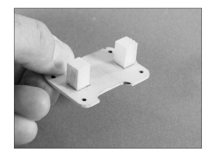
○ ○ 11. Use a pin drill and 1/16-inch (1.5mm) drill bit to drill the two mounting holes for the servo in the blocks.
