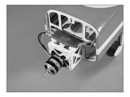
• 4. This photo shows the installation of the 480 motor. Simply follow Steps 1 through 3, only using the 480 motor instead of the 450 motor.
