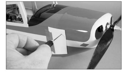
*Note*: Ensure the painted stripe on the cowl lines up with the stripe on the fuselage
