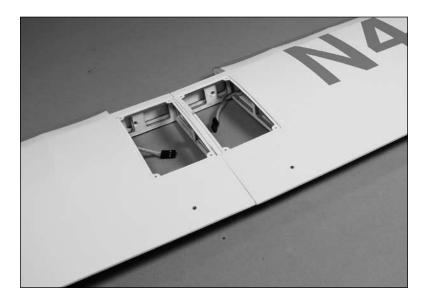
• 6. Mix around 1/2 oz (15ml) of 30-minute epoxy. Apply epoxy to the joiner, including any edges that will come in contact with the wing panel when it is installed.
