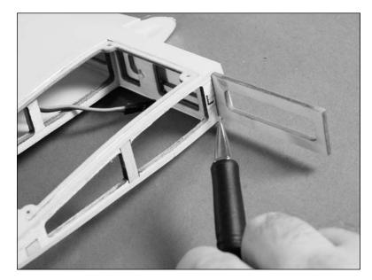
• 4. Slide the joiner into the other wing panel. It should slide in the panel up to or farther than the line drawn in the previous step. If not, sand the end of the joiner so it will slide in at least up to the line.
