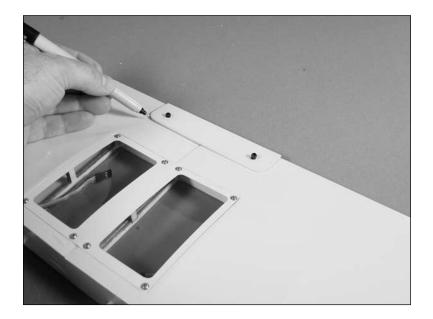
*Hint*: Use two of the 4-40 bolts through the holes in the brace and wing to keep it in position while tracing it with the pen.
