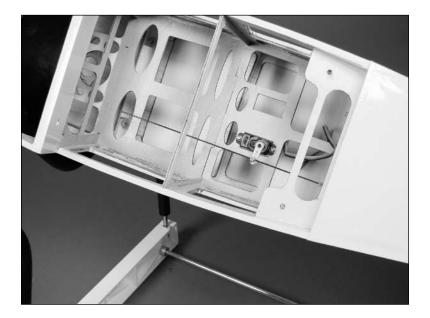
• 7. Repeat Steps 1 through 6 to install the elevator pushrod and servo.
