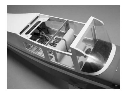
5. Test fit the struts between the fuselage and wing. The strut end will slide under the landing gear covers as shown. They can be turned over (top to bottom) if they do not align with the holes in the wing and fuselage. Secure the strut to the fuselage using a 2mm x 8mm sheet metal screw.
