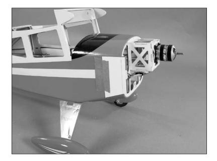
• 7. Slide the cowling onto the fuselage.
