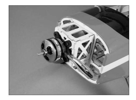
• 5. Turn on the radio system and plug the battery into the speed control. Use the throttle to check that the motor rotates counterclockwise when viewed from the front. If not, follow the directions included with your speed control to change the direction of the motor rotation.
