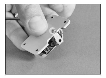
○ ○ 9. Use a pencil to mark the location of the servo mounting tabs on the plate.
