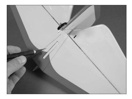
• 6. Slide the dowels in the wing in the holes of the fuselage.
