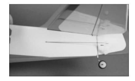
$\bigcirc$   $\bigcirc$  3. Insert the control horn into the slot in the rudder.
