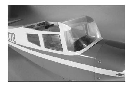
• 4. Use canopy glue to secure the seats inside the fuselage. Allow the fuselage to rest on its wheels until the glue fully cures.
