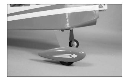
• • • 7. Use a felt-tipped pen to mark the location for the wheel pant screw.
