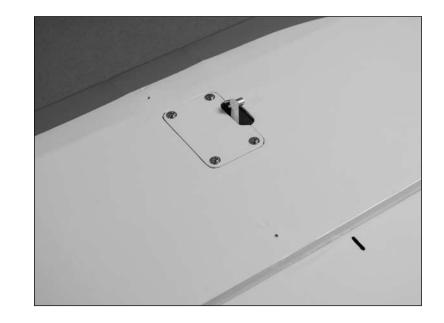
○ ○ 17. Use 6-minute epoxy to glue the aileron servo horn in position. Make sure to press the horn fully into the slot in the aileron.
