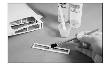
• 7. Apply epoxy inside the opening in the wing as well.
