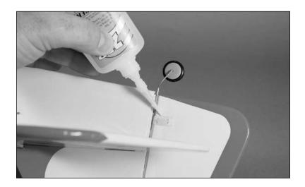
○ ○ 6. Attach the micro pushrod connector to the servo arm using the same technique used for the aileron servo. Mount the rudder servo using the hardware provided with the servo. After centering the servo, secure the pushrod using a 2mm x 4mm machine screw and #1 phillips. Use side cutters to trim the pushrod wire to the correct length.
