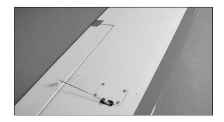
○ ○ 21. With the radio on, check the operation of the aileron servo again. Use a 2mmx 4mm machine screw and a #1 Phillips screwdriver to secure the pushrod to the connector. Use side cutters to remove any excess wire extending beyond the connector.
