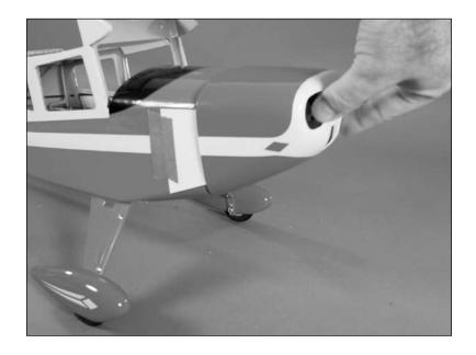
• 8. Attach the propeller to the adapter and slide the assembly onto the motor shaft.
