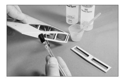
• 9. Use medium CA to glue the wing dowels in position. They will slide in the wing until they are flush with the back side of the wing center section.
