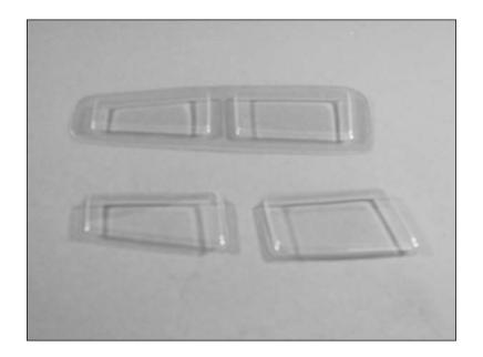
• 2. Use canopy glue to glue the window in from the inside of the fuselage. Use low-tack masking tape to hold the windows in position until the glue fully cures.
