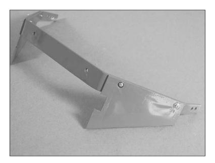
• 2. Attach the landing gear to the fuselage using two 4-40 x 3/8-inch socket head screws and two #4 washers. Use threadlock on the screws to prevent them from vibrating loose in flight.
