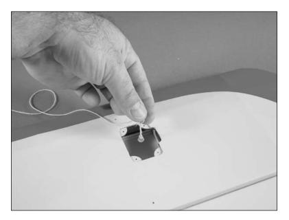
• • • 14. Tip the wing up and allow the weight to drop to the center of the wing.
