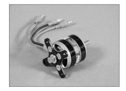
• 2. Attach the motor to the motor box using four 4-40 x 3/8-inch socket head screws. Use threadlock to prevent the screws from vibrating loose during flight.
