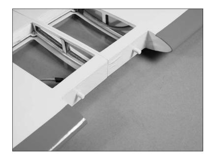
10. Attach the skylight to the wing using eight 2mm x 6mm sheet metal screws using a #1 Phillips screwdriver. Leave the screws slightly loose until they have all been started so you can adjust the position of the window.
