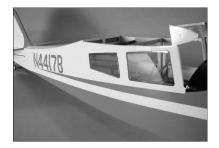
• 3. Use canopy glue to glue the windshield to the fuselage. Use low-tack masking tape to hold the windshield in position until the glue fully cures.
