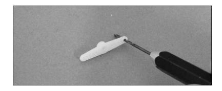
○ ○ 2. Slide a micro pushrod connector into the hole drilled in the previous step.
