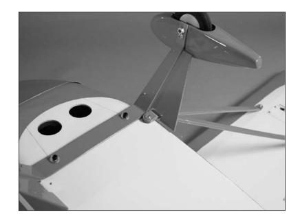
• 6. Secure the struts to the wing using two 2mm x 8mm sheet metal screws.
