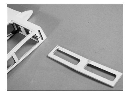
• 2. Slide the wing joiner into the wing panel. It may be necessary to sand it lightly for the best fit.
