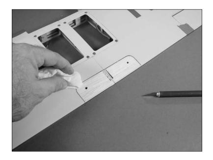
• 16. Use medium CA to glue the brace to the wing. Hold the brace tightly against the wing until the CA cures.
