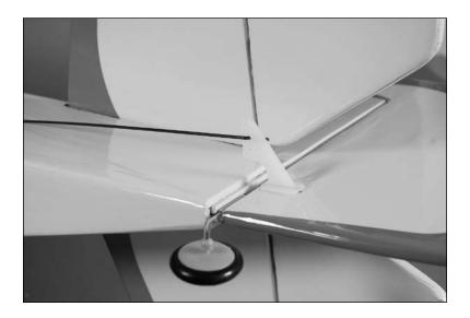
*Hint*: Use low-tack masking tape to hold the rudder and elevator centered while installing the servos.
