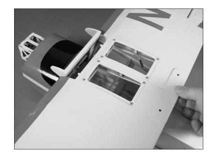
• 7. Secure the wing to the fuselage using two 4-40 x 1-inch socket head screws and two #4 washers.
