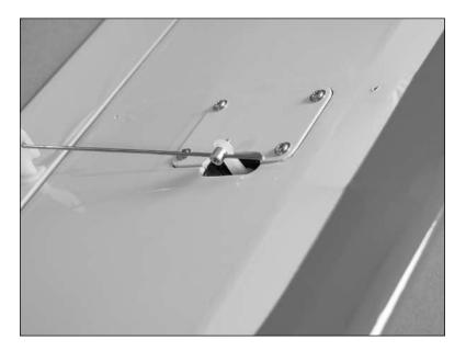
Q Q 20. Use a piece of low-tack tape to hold the aileron in neutral. You can leave the tape in place until you are ready to set the control throws to help prevent moving the aileron and possibly stripping the servo gears.
