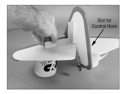
*Hint*: Rest the stabilizer on two coffee cups. This will suspend the assembly and keep the tail wheel from causing any issues with keeping things square.
