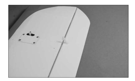
○ ○ 18. Attach the 3<sup>3</sup>/<sub>4</sub>-inch (95mm) aileron pushrod to the middle hole of the control horn.
