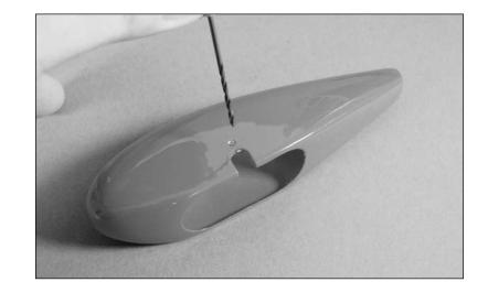
○ ○ 9. Position the wheel pant back on the gear and secure it using a 2mm x 6mm sheet metal screw.
