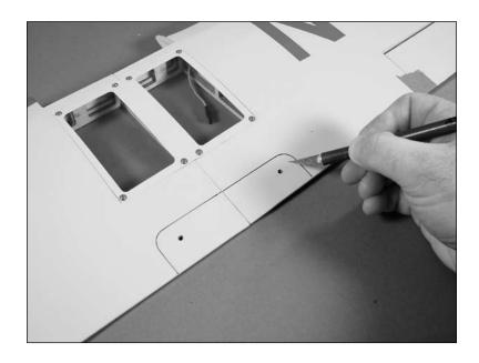
**Note**: Use light pressure to avoid cutting into the underlying structure. A soldering iron of hot knife can be used as an option, reducing the chances of cutting into the wood.
