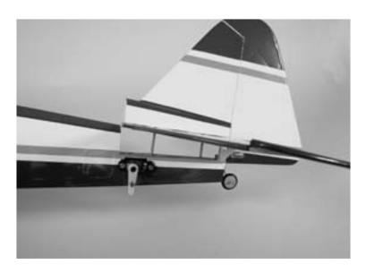
3. Slide the #4 washers onto the threaded rods. Thread the nuts onto the rod, tightening them snugly against the bottom of the fuselage.
