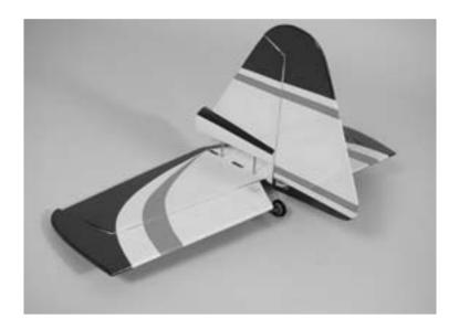
2. Slide the rudder/stabilizer assembly onto the fuselage.
