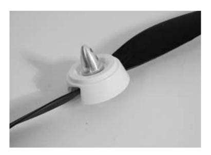
4. Install the propeller assembly onto the motor shaft. Tighten the propeller nut using a hex wrench slipped through the hole in the propeller nut.
