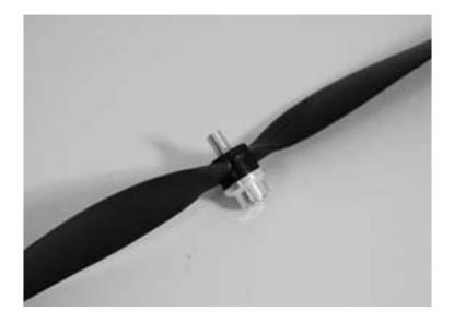
2. Slide the 1/2" (13mm) washer onto the adapter.
