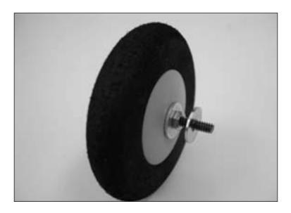
3. Fit the assembly in Step 2 into the wheel pant and insert the bolt into the landing gear. With the fuselage level to the work surface, rotate the wheel pant so it is also level to your work surface and secure the pant to the landing gear with a 2mm x 6mm wood screw. Secure the bolt with a 4-40 locknut while using needle-nose pliers to hold the head of the bolt inside the pant.
