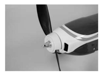
**Note**: Make sure to check the balance of the propeller after enlarging the hole in the propeller.
