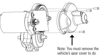
Gear mesh has already been set at the factory, and setting it is only necessary when changing motors or gears.
