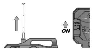
3. Do a Test of Transmitter's control of vehicle with vehicle wheels off ground
