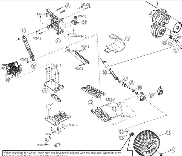
hex is removed, the drive pin can fall out of the axle.
