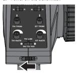
4. Remove the battery from the vehicle.
