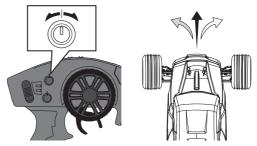
**IMPORTANT:** Seat the motor brushes by driving smoothly on a flat surface during use of the first battery charge. Properly seating the motor brushes will increase the life and performance of the motor.
