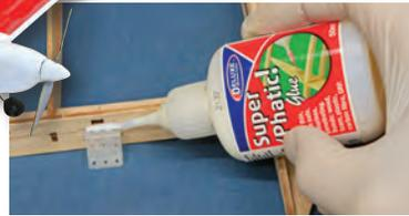
1. Just apply a small bead of Super'Phatic! to your hinge & slide it into the wing. It will be dry & ready to go in only a few hours.
