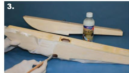
Fig 3. Eze-Kote is then brushed through the glass fabric. The float in the background has already been covered.
