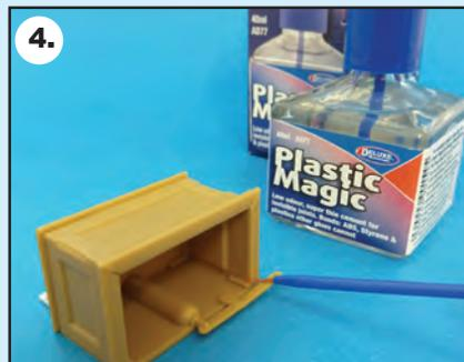
Fig 4. Use **Plastic Magic** to assemble the toilet cistern & create a nice strong bond.
