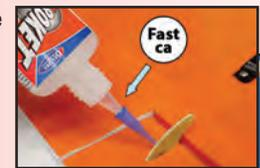
Here, the outer trailing edge of a balsa wing rib needed to be glued to a tiny notch in the wing trailing edge. A drop of **Rocket Hot** applied to the joint did the job in two seconds.
