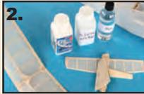
**Fig 3.** This solution was brushed onto the frame with a soft head brush which seals the tissue in place.
