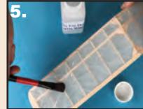
**Fig 6.** As a diesel engine was being fitted we doped the engine bay with **Eze Dope** solution which renders the surface 100% fuel proof.
