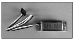
An optional DigitalTachometer (DLEG5525) is available that can be directly connected to the ignition and display the RPMs of the engine. This unit can be installed on the aircraft or used to spot check the Engine RPMs. Do not install
