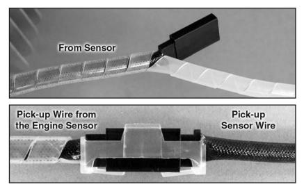
**2.** Install the silicone wire cover over the pick up lead coming from the engine (cut the excess silicone wire cover) and connect the lead to the pick–up lead from the Electronic Ignition Module. Secure the connection with the included three pin connector securing clip.
