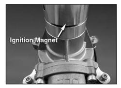
**3**. Next, set the engine at the beginning of the compression stroke. Note the position of the ignition magnet.
