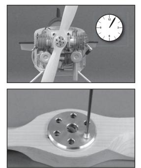
**4**. Place the propeller on the crankshaft at the one o'clock position.
