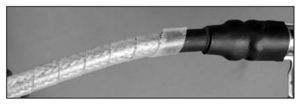
7. Install the remaining silicone wire cover over the ignition wire.
