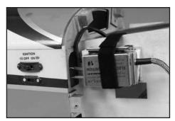
6. Install the ignition module and battery securely in the airplane forward area. It is recommended that a thin piece of foam rubber is placed between the module and the mounting surface and that Velcro<sup>®</sup> strap is used to hold the module in place.
