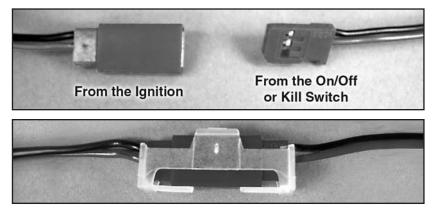
**3.** Connect the manual on/off switch lead to the red connector from the electronic ignition system using the lead from the kill switch or with the included three pin connector with pig tail. Use one of the included three pin securing clips to secure the connection.
