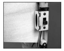
**4**. Install the manual on/off switch on the aircraft so that it is easily accessible from outside the plane.
