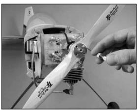
5. Mark the location of one of the outer holes while the propeller is in the beginning of the compression stroke position. Use a GPM Dead Center Hole Locator (GPMR8130) to center and start the hole.
