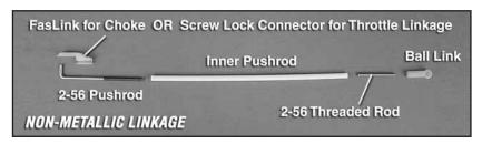
5. Install the choke servo (optional) at least 12" [305 mm] away from the engine. Be sure to use a non-metallic linkage.
