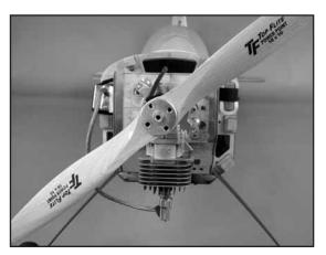
**4.** Place the propeller on the crankshaft at the one o'clock position.
