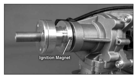
**3.** Next, set the engine at the beginning of the compression stroke. Note the position of the ignition magnet with engine inverted.
