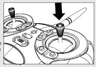
By pushing in on the right-hand stick while in the high-rate mode, you can enter the low-rate mode. You can tell you are in the low-rate mode when the LED on the transmitter blinks continuously. The low-rate mode is typically preferred by (and best for) first-time, low-time and other pilots interested most in a reduced amount of control that allows for smoother and more easily controlled hovering and flying.
