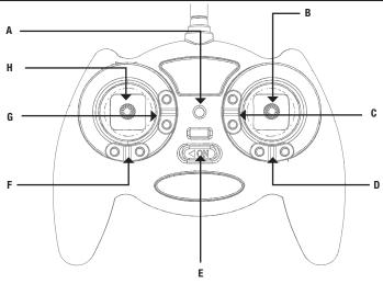
**NOTICE:** When pressed down, trim buttons make a sound that increases or decreases in pitch at each pressing. The middle or neutral trim position is heard as a middle tone in the pitch range of the sounds. The end of the control range is sounded by a series of beeps.
