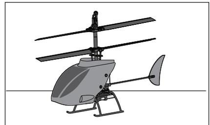
Put the helicopter on a flat, level surface. The helicopter gyro stabilizes at this time. Do not allow the helicopter to move until the red LED on the helicopter is solid.
