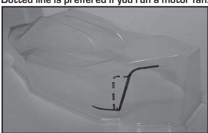
Install hook and loop tape (#91743) along the side braces in 2 spots.
