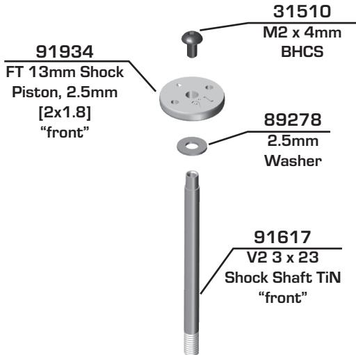
! Mount the shock pistons with the number facing up!
