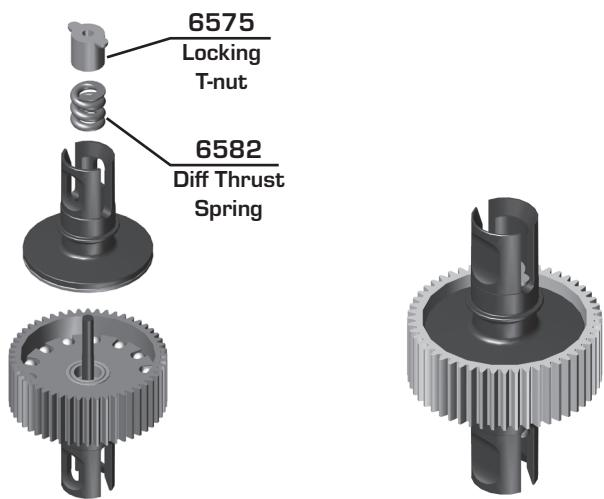
As you tighten the diff bolt, you will notice the T-nut ears moving closer to the bottom of the outdrive slot. This compresses the spring behind the T-nut. The spring should be completely
