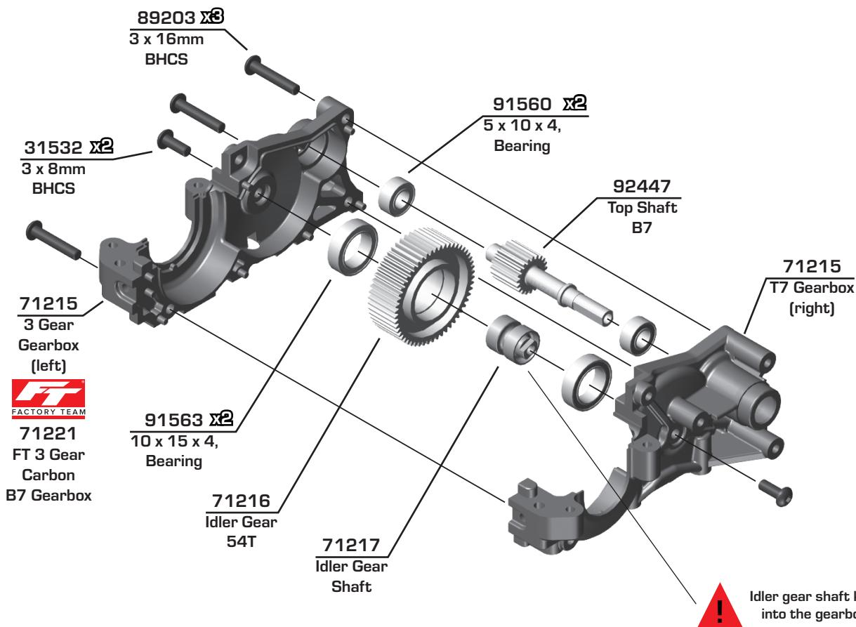
! Idler gear shaft keys into the gearbox.
