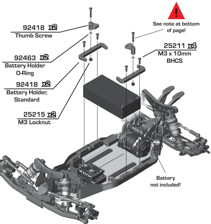
Standard and Low Profile battery thumb screws are included. Shims may need to be added if battery weights are used.
