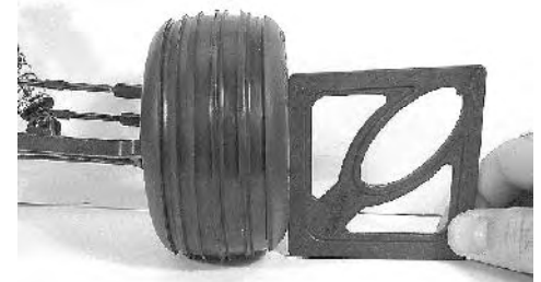
Testing camber with the camber gauge
