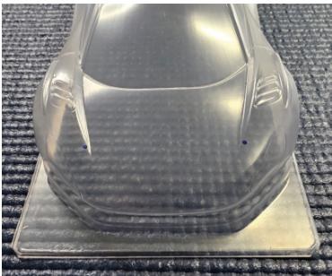
2. Mark rear body post holes – 2.5mm further forward (from center) than existing rearward most dimples.
