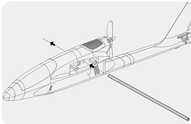
2. Apply the left and right wing halves onto wing spar, pass the servo wires into fuselage and then have them connected with a 2Y harness.
