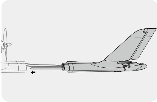
2. Secure the joint of the front and rear fuselage using included screw.
