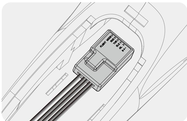
2. Tear off the adhesive sticker on the back of Vector unit and stick the Vector unit to the position as shown in the below figure.
