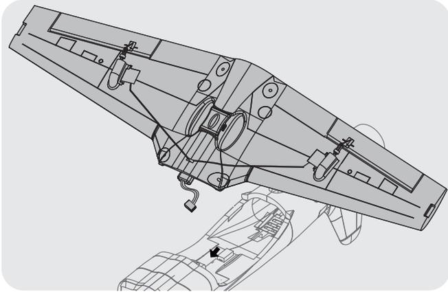
2. Attach the wing to the fuselage using the included screws.
