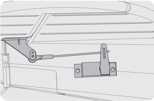
2. With the servo and rudder centered, connect the servo to the control surface using a pushrod.
