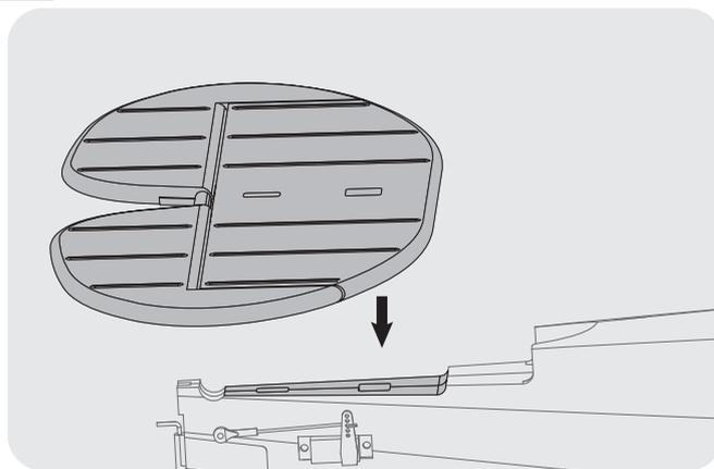
2. Place the vertical stabilizer onto the horizontal stabilizer. Secure using the included screw.
