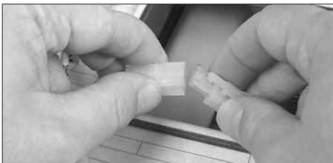
❑ 2. Plug the battery pack into the boat’s ESC (Electronic Speed Control) battery connector. Do not force them together; they are designed to fit together only one way.
