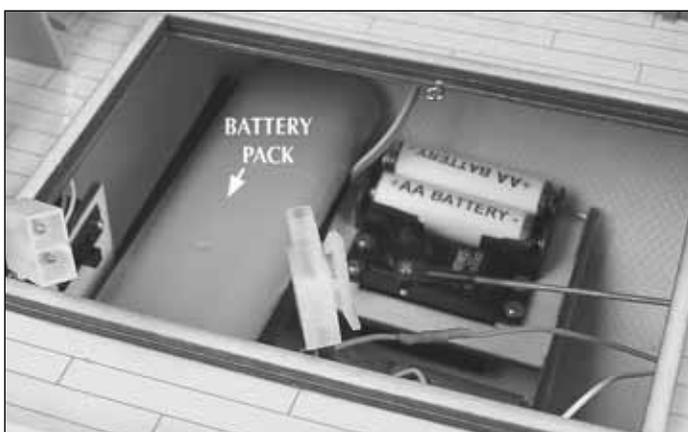
❑ 1. Peel the backing off of the supplied hook & loop material and apply the “loop” side to your 6-cell battery pack. With the cabin removed from the deck, place a fully charged battery pack onto the battery tray as shown.
