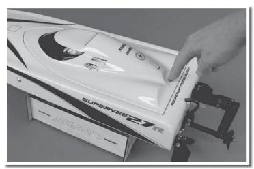
Install the cowl and snap it in place by pushing down on the back latch. You are now ready to run the boat.
