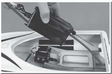
7. Slide the box forward, slipping the water pickup line and rudder push rod out of the boat as well. Lift the box out and set aside.
