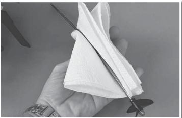
2. Firmly pull the prop and drive shaft out of the back of the boat. Wipe away any old grease and water.
