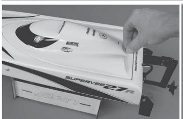
3. Remove the hook and loop from the battery area inside the boat and attach it to your battery packs.
