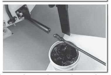
3. Apply new speed grease to the shaft and slide it back into the strut, moving it in and out as you do so to help spread the grease along the length of the cable.
