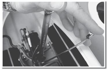
1. Loosen the cable coupler using the 10 and 12mm wrenches.
