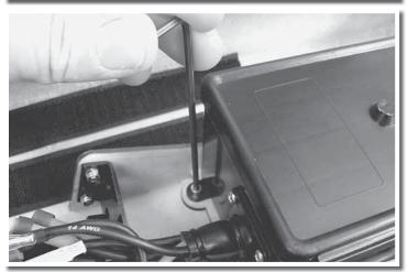
6. Use a 2.5mm ball driver or hex wrench two remove the two M3 screws holding the radio box in place.
