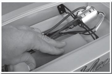
Stand clear of the propeller and plug each of the battery packs into the motor controller.
