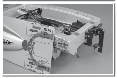
At the end of the day make sure to leave the cowl off and the drain plug out overnight. This will allow any moisture that collected in the boat to safely evaporate.
