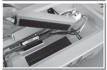
Install the batteries, making sure they are well seated.
