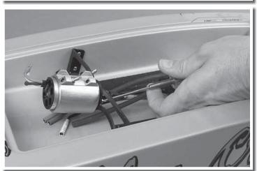
Remove the motor from the boat.
