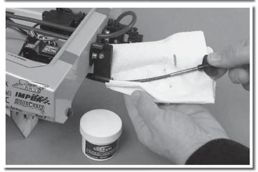
After each 5 or so runs and/or after a day of running it's a good idea to re-lubricate the drive cable. Loosen the cable coupler using the 10 and 12mm wrenches. Firmly pull the prop and drive shaft out of the back of the boat. Wipe away any old grease and water. Apply new speed grease to the shaft and slide it back into the strut, moving it in and out as you do so to help spread the grease along the length of the cable.
