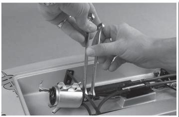
Fully loosen the coupler. Using a rag cover the prop and firmly pull the prop and shaft away from the coupler. Use a 2.5mm hex wrench to loosen the two motor screws.
