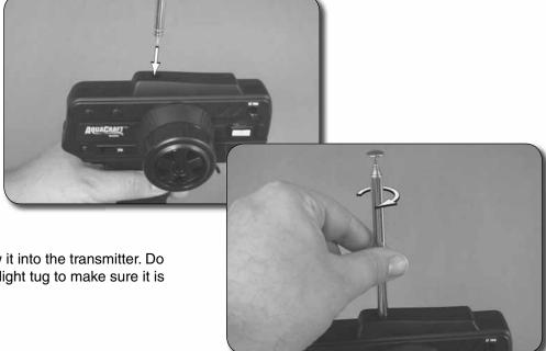
2. Slip the antenna in and gently screw it into the transmitter. Do not overtighten. Give the antenna a light tug to make sure it is properly installed.
