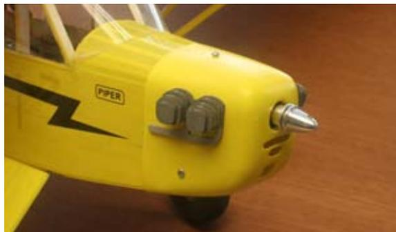
119...Cut the paper cooling shrouds from the plan. Paint them black. Bend them to shape and glue to the cowl and parts M-6.
