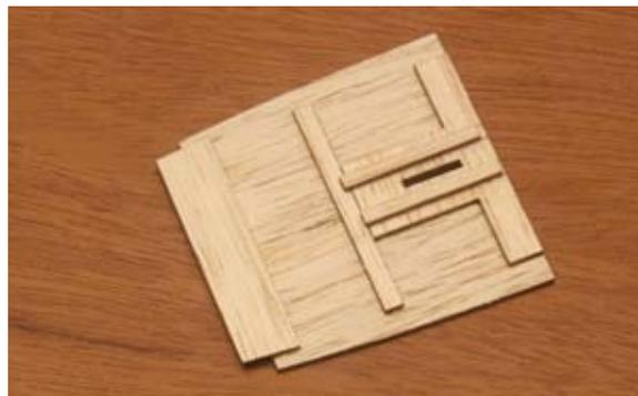
25...With the H-5/6 slider in position, carefully glue the two H-8 pieces into position. Use the tip of a straight pin to apply a tiny amount of glue to the outside edges of the H-8's. Use extreme care to make sure that you DO NOT glue the H-5/6 slider into position!!!
