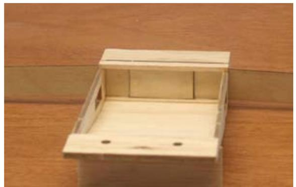
44...Sheet the bottom of the center section with the 1/16" sheet as you did the top.
