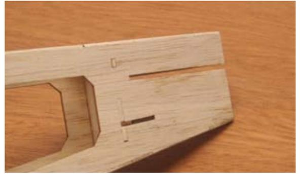
30...Test fit the tail surfaces on the fuselage. Trim and sand if needed to achieve the proper fit. Cut the bottom rudder hinge slot in the end of the fuselage.
