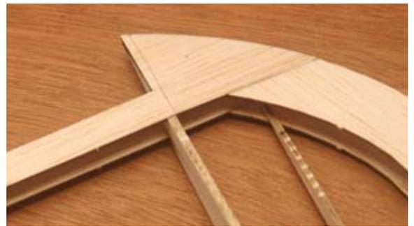
64...Lay the wing upside down on your building board. Hold it so it is level front to back and the top spar is in contact with the building board.
