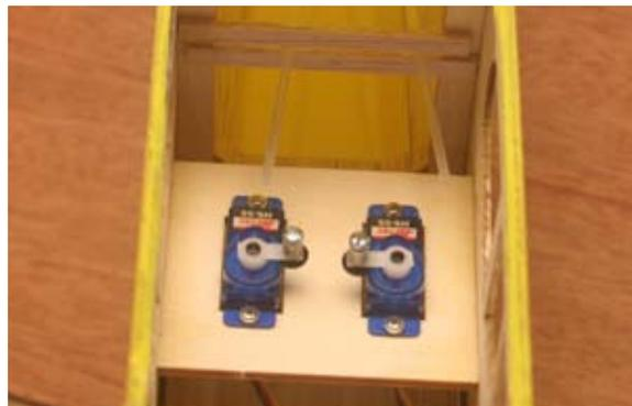
94...Install the pushrods into the housings. Secure the rear of the pushrods with Mini E/Z Links.
