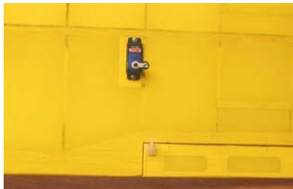
107...Install the pushrods. Attach the rear of the pushrods to the horns with Mini E/Z Links. The front ends are attached to the servos with Mini E/Z Connectors. When the servos are in neutral the servo arm should be 30 degrees forward as shown.
