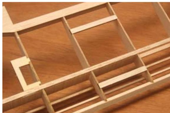
70...Cut four pieces 1 1/2" wide from the 1/16" x 3" x 12" balsa sheet. Use them to sheet the top and bottom center of the wing. The sheet should be cut to fit between the spars as shown on the plan.
