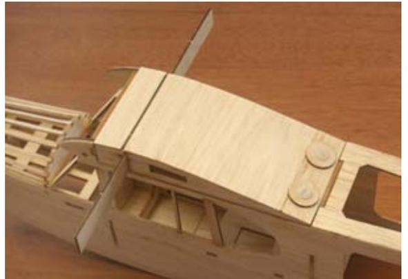
48...Glue W-23 into position on the sheet on the bottom of the center section. Cut away the sheet from the center when the glue dries.
