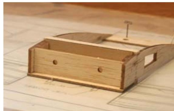
38...Glue the second W-14A into position on the front of the previous one. Now glue W-14B into position on front of the W-14A's.
