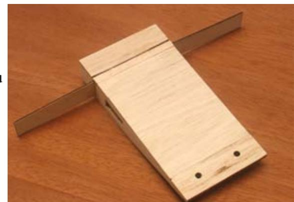
45...Cut two pieces from the 1/8" dowel approximately 3/4" long. Insert them into the holes in the front of W-14B. They should stick out just over 1/4". Securely glue them into position.
