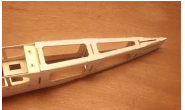
19...Glue F-20 into position on the bottom of the fuselage.
