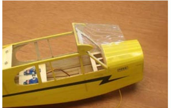
Cut the windshield to the pattern on the plan. Tape it down at the top of F-6. Wrap it around and tape the lower rear corners to the fuselage sides. Mark and trim as required. Now glue the windshield to the model with thin C/A. Start at the top. When this is dry work your way slowly around the rest of the windshield.
