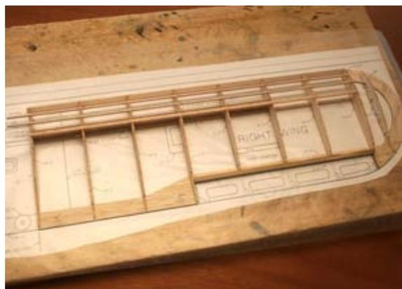
59...Glue the top trailing edge / wing tip parts W-16, W-17 and W-18T together.
