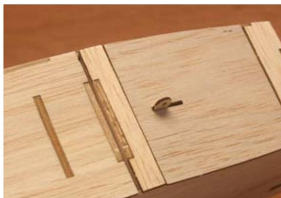
28...Use a sanding block to sand all of the fuselage surfaces smooth all over. Now lightly sand the corners of the fuselage round. Leave the wing opening square.
