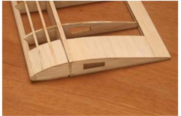
72...Sand the leading edge of the wing round to match the profile shown on the plan. Sand the trailing edge and wing tip round. Leave the edges of the aileron cutout square. Now sand the wing smooth all over.
