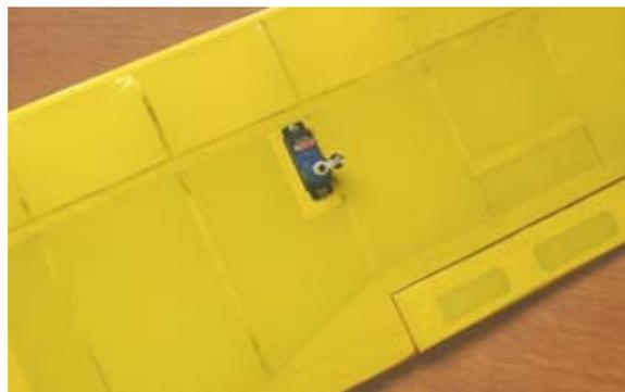
106...Glue the aileron control horns into position on the bottom of the ailerons. Drill 1/16" holes for the pins to fit into.
