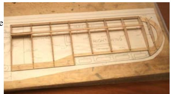
56...Glue two W-19's together. Put into position and glue to the ribs and the trailing edge.
