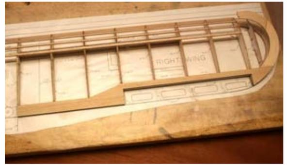
61...Roll the front of the wing tip forward and glue to W-9 and W-10. The very end of the wing tip should be level with ( the same height ) as the main spar at rib W-9.
