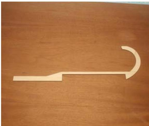
60...Glue the top trailing edge / wing tip into position, Glue it to ribs W-1 thru W-9 and the back of W-10.
