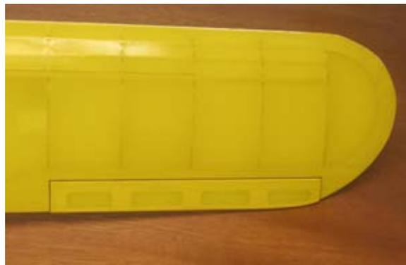
105...Screw the servos into position on the bottom of the wing.
