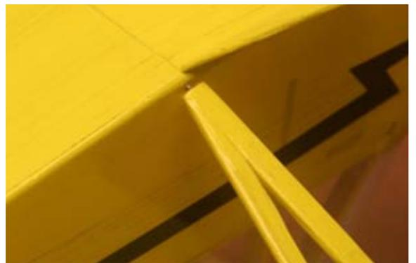
112...Place 1/2" pieces of aluminum tube over the wires at the outboard ends of the wing struts. Place the ends of the struts on the bottom of the wing over the W-21's. Adjust the bends on each end of the struts so the tubes lay flat on the bottom of the wing. Mark the location of the tubes on the wing. Remove the struts and glue the tubes to the bottom of the wing. Reinstall the struts to check the fit.
