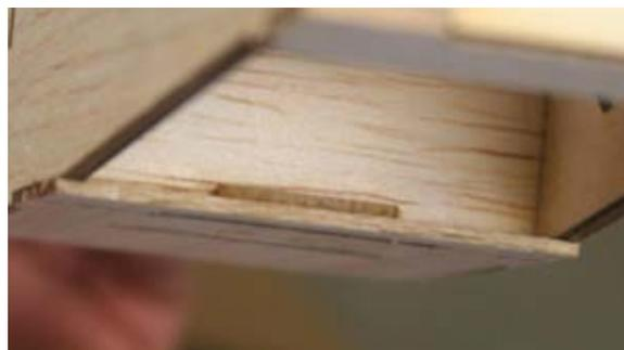
27...Test fit the hatch to the bottom of the fuselage. The front tab (H-2) slides under part F-13. Slide the hatch slider forward and press the back end of the hatch down on the fuselage. Move the slider back to secure the hatch. Trim the 1/16" spacer as required to allow the slider to move to the rear. You can trim the outside edges of H-2 to center the front of the hatch if required.
