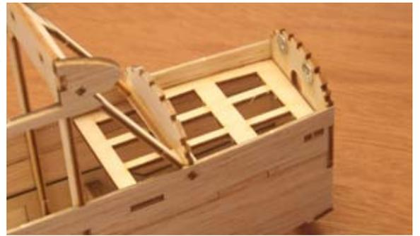
21...Using the 3/32" sq. X 18" strips, glue the stringers to the top front fuselage between F-11 and F-21. Trim the stringers flush with the formers.
