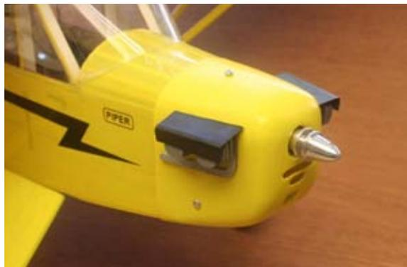
120...WITH THE PROPELLER REMOVED...Turn the transmitter on. Place the throttle stick in the low position. Plug the battery into the speed controller. Check the motor for proper operation and direction of rotation. Follow the instructions with the speed controller to make any adjustments.
