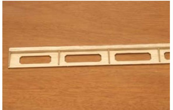
77...Glue A-1T onto the top of the aileron. Sand the ends, front, top and rear of the aileron flush.
