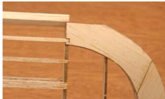
67...Glue two W-22's into position against the top and bottom sheet and the 1/4" sq. leading edge.
