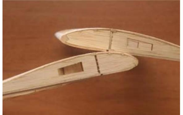
83...Slide the wing joiner on the center section into position in the right wing. Position it tightly between the spars and forward against the shear web and glue the right wing to the center section.
