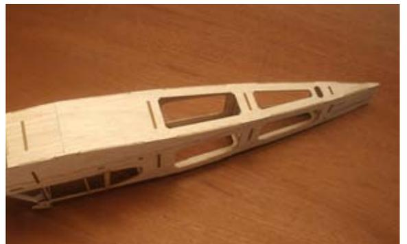
20...Glue former F-21 into position on the top front of the fuselage. It should be centered left and right, be 90 degrees to the top of the fuselage and be touching former F-9.
