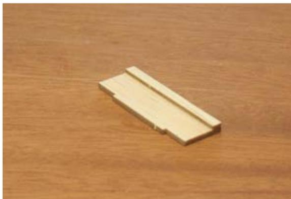
12...Glue the other F-14 in place. Use a small scrap of 1/16" balsa to space the F-14's apart at the open end. Do not glue the spacer.
