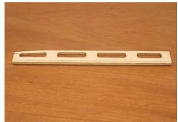
80...Mark a line on the back of the aileron spar (W-19) 1/8" down from the top. Mark the hinge locations and cut slots for the hinges. Temporarily install the hinges and check the aileron for proper fit on the wing. Do not glue the hinges at this time.
