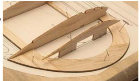
55...Glue the 3/32" x 3/16" top spar into position. The spar stops at the W-9 rib. Glue the 1/4" sq. leading edge into position in the notches in the front of the ribs. The leading edge stops at rib W-9. Be careful to not allow glue to run down onto W-18.
