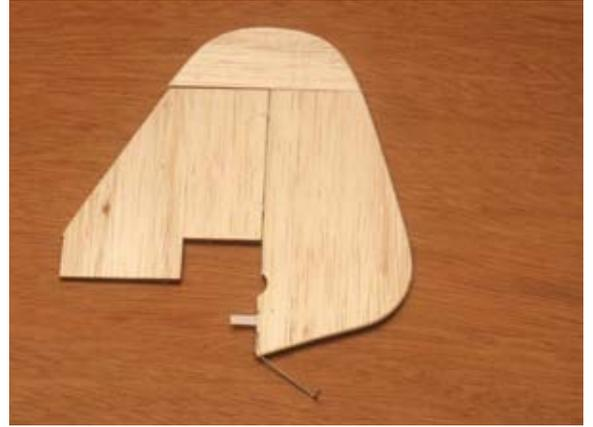
2...Sand the 1/8"x 3" dowel to 3/32" diameter. Join the elevators (S-2) using this dowel. Use the stabilizer as a guide. Trim the dowel if required to achieve the proper length.
