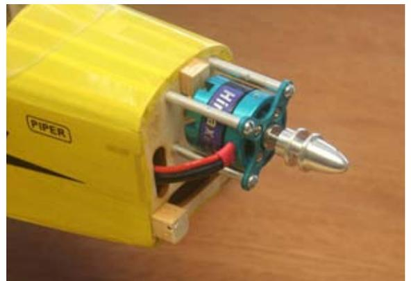
118...Place the cowl in place. Drill 1/16" holes thru the cowl and mounting blocks. Secure the cowl to the model with the #2 X 1/2" sheet metal screws.
