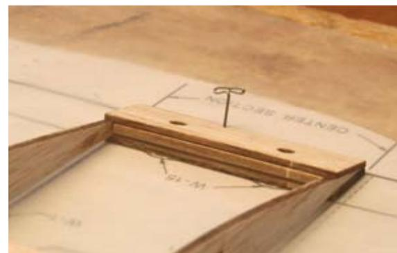
40...Use the 1/16" x 3" x 12" balsa sheet to sheet the top of the center section. Cut the sheet so the grain runs left to right. The sheet should but up against and be flush with W-11 and the spar. The front piece rests on top of the F-14's.
