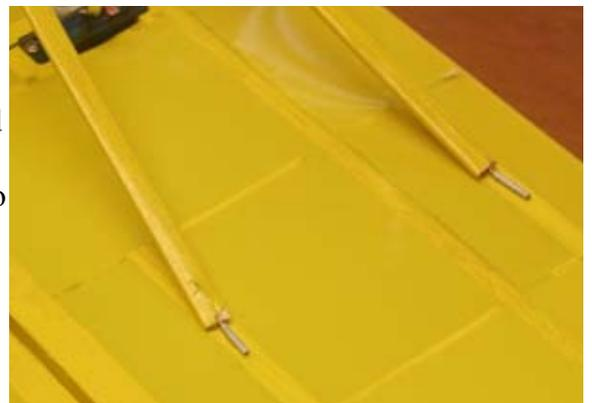
113...Glue two 1" long pieces of 3/32" sq. balsa into the holes in M-1. They should be 90 degrees to M-1.
