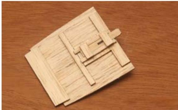
26...Glue a small scrap of 1/16" sheet about 1/2" square for filler to the inside of F-15. The front end should be trimmed off flush with the front of F-15.
