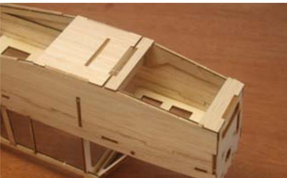
15...Place former F-17 into position and pull the rear of the fuselage sides together. Adjust the back end until the fuselage is straight and square. Glue the fuselage sides together and glue the former in place.
