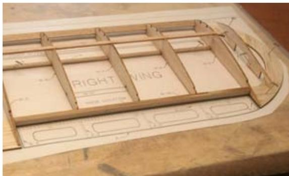
57...Glue the remaining shear webs ( C thru F ) into position. Trim the ends to get the proper fit if needed.
