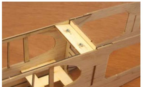
10...Glue F-13 into position on the bottom front of the fuselage.
