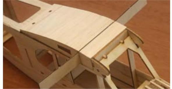
47...Place the W-15 discs onto the nylon screws and thread them into place. Glue the W-15's to the top of the center section.
