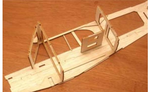
7...Place the left fuselage side into position and square up the fuselage. Glue the left fuselage to the formers. Make sure that the fuselage is square and completely glue the formers to the fuselage sides.
