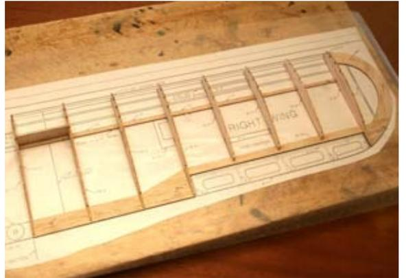
54...Pin the W-10 rib into position on the plan. The standoffs should be placed on the hatched areas on the plan.
