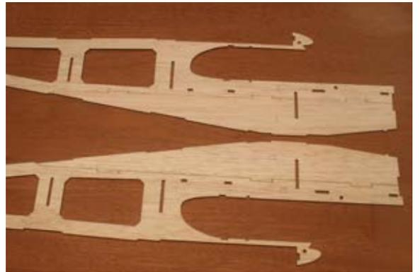
4...Glue the F-2 and F-3 doublers to the inside of the F-1R & F-1L fuselage sides. Be sure to make a right hand and a left hand side.
