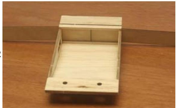
43...Center W-12A on the back of the joiners and glue into position.
