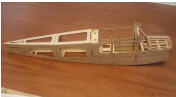
29...Cut away the wood from the stabilizer slot between the dashed lines.
