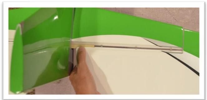
Apply petroleum jelly (Vaseline) to the center hinge pin portion of each hinge. This will help prevent glue from getting into the hinge when gluing then into the elevator. Avoid getting petroleum jelly on the barbed portion of the pin. If you do clean it off with alcohol.
