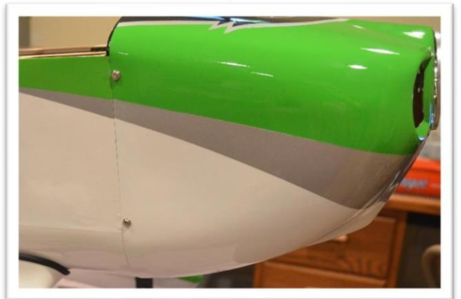
Remove the cowl and apply thin CA glue to the mounting tabs and screw holes. (Allow plenty of time for the CA glue to dry before reinstalling the cowl.)
