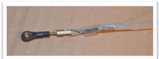
Connect the ball links to the rudder control horn using a socket head screw, nylon lock nut and a washer. Pull the slack out of the cables and make sure the cables cross once inside the fuselage.
