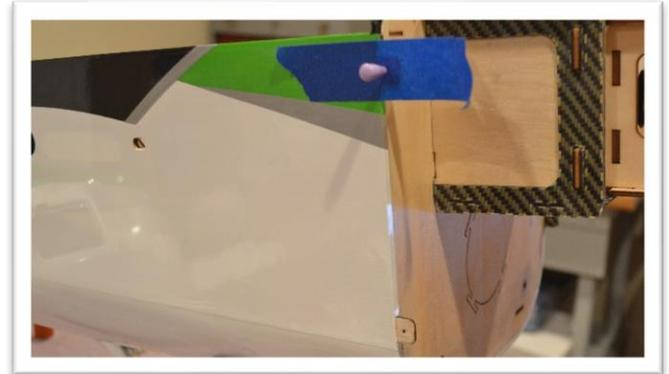
Peel back the tape to uncover the mounting tabs and install the cowl but leave the tape on the fuselage. Tape the cowl into position centering it to the motor using your spinner's back plate as a guide and aligning it to the top edge of the firewall.
