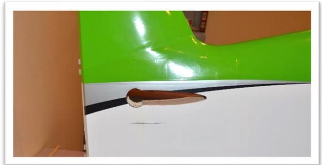
Review the servo configurations as described on page 4 before cutting the covering over the servo pockets. Below the horizontal stabilizer slot there is a servo pocket on each sides of the fuselage. Cut only one of them open if you plan to use 1 elevator servo. Cut one open on each side if you plan on using 2 elevator servos. Use a sealing iron to attach the covering around the opening before cutting.
