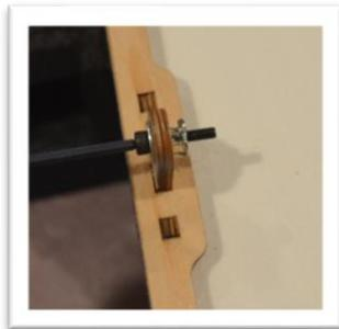
Secure the canopy to the fuselage with the 3mm thumb screws and flat washers.
