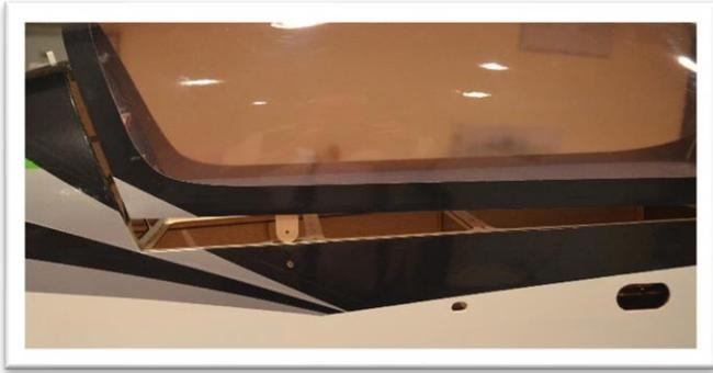
Enlarge the hole in the canopy mounting tab to receive the 3mm blind nuts. Use a washer and machine screw to draw the blind nut into the canopy mounting tab.
