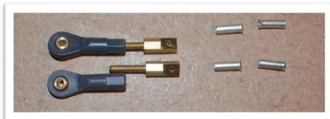
Start the cable assembly at the servo end inside the fuselage. Thread on 2 crush sleeves and the brass cable eye. (Many people also thread on some heat shrink tube to cover the assembly to give a finished look.)
