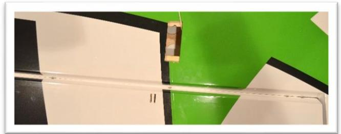
Use the control horns from the "Wings" part bag. Test fit the control horn in the slot. Trim or file the slot as needed to achieve a snug fit. Make sure the shoulder of the control horn is fully seated down against the control surface.
