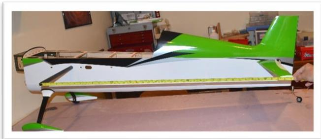
Once the horizontal stabilizer is positioned glue it in place with thin CA glue. Wick glue in on both sides, top and bottom. The use of an applicator tip is suggested to control the flow of thin CA and get it exactly where you want it.
