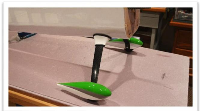
Ensure all set screws are tight on the pre-assembled tail wheel assembly.
