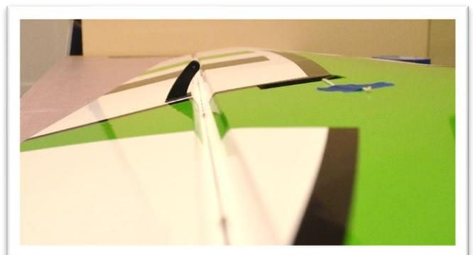
With the control horn in position apply painter's masking tape around the control horn base. Put the tape up to the base edge. Not under or over it.
