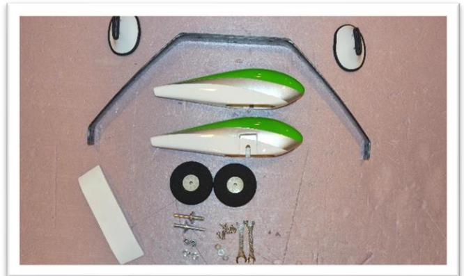
Use the landing gear fasteners (4mm) located on the bottom of the fuselage along with 3 flat washers located in the landing gear package to assemble the landing gear. Add a drop of removable thread locker to the screws during assembly.
