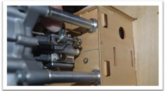
The placement of the throttle servo is dependent on the engine you choose to use. The servo can be mounted in the front of the fuselage in many cases. (If you choose this location drill 5 holes through the top of the engine box so servo mounting screws and the servo arm screws can be accessed.)
