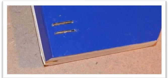
Test fit the control horn halves in the slot individually, then as an assembly. The fit should be snug.
