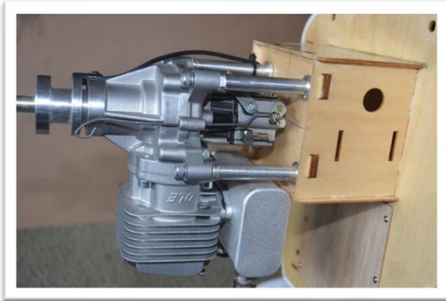
Bolt the engine standoff to the firewall from the back.
