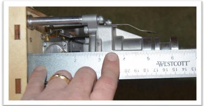
Check for clearance between the firewall and the carburetor. This distance should be noted in your engine's manual. If you don't have at least the recommended space cut an opening in the firewall so the carburetor can get air.
