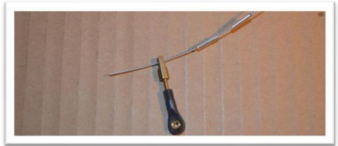
Loop around the cable eye and go back through the first crush sleeve.
