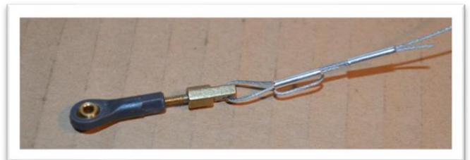
Adjust the loops and crimp the sleeves with the non-serrated surface plyers.
