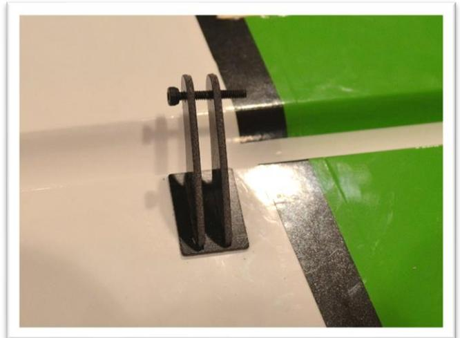
Check the alignment of the control horn to the hinge center line. The linkage hole in the control horn should be aligned with the hinge centerline.
