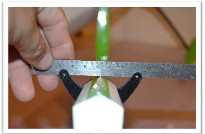
Use 30 minute epoxy to glue the control horns in place. Check the alignment, peel the masking tape away and set aside for the epoxy to cure.
