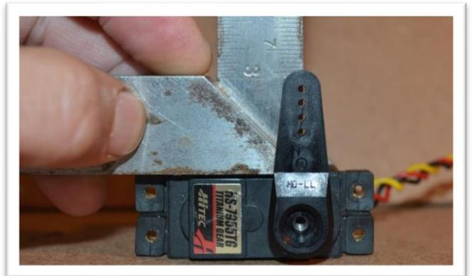
Install the servo into the fuselage and pre-drill for servo mounting screws using a 1/16" drill. Install the servo with the wood screws that came with your servos. Remove the screws and servo. Apply a drop of thin CA glue into each screw hole. This will harden the wood around the screws and provide a more secure installation. (Allow the CA glue to dry before reinstalling the servo.)
