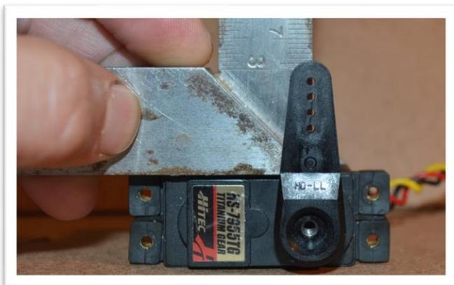
Attach the servo wire to the installation string and gently pull the wire through the wing as you insert the servo into the wing. (Depending on the length of the servo wire provided it may be necessary to install a servo extension wire before installing through the wing.)
