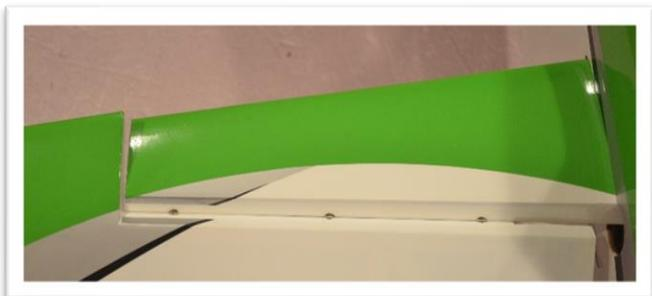
A small round file can be used to give the hinges some clearance. Cleaning out the holes will also help you close up any gap. Turn a 1/8" drill into the holes by hand.
