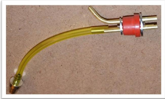
Insert the assembly into the fuel tank and check that the clunk is free to move around. Rotate the tank side to side and upside down to ensure the clunk does not get stuck. If cluck does not move freely in all positions trim a little off the fuel line and try it again. When you have established the correct length of the fuel line you can tighten the stopper screw.
