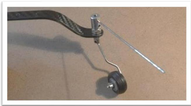
Use the landing gear fasteners (4-40) locate on the bottom of the fuselage along with 2 flat washers located in the landing gear package to mount the carbon fiber landing gear. Add a drop to removable thread locker to screws during assembly.
