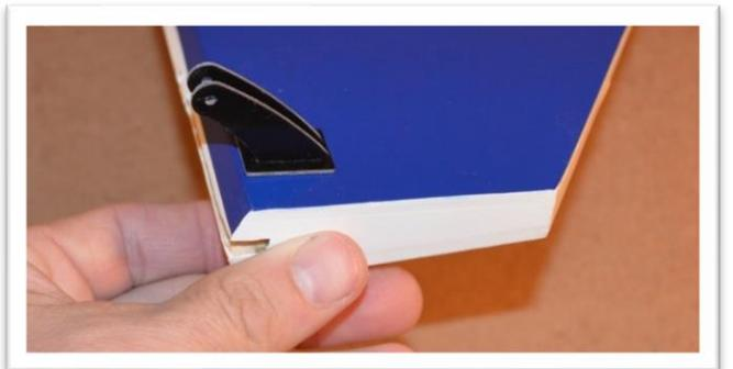
With the control horn in position apply painter's masking tape around the control horn base. Put the tape up to the base edge. Not under or over it.
