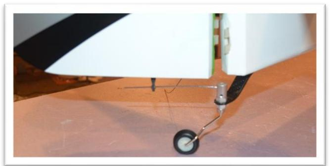
Align the rudder hinges to the vertical stabilizer hinges. Insert the rudder hinge pin through the top of the rudder then through each of the hinges.
