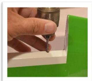
Test fit pieces together and adjust as needed so you get a good fit between the elevator and the stabilizer. Check the hinge gap and the gap at the counter balance. Make sure there is clearance between the elevator jointer plate and the fuselage. Hold half of the elevator aligned to the leading edge of the stabilizer and ensure the opposite elevator half is also aligned. Sand or shim the elevator jointer plate until both halves are aligned to at the leading edge of the stabilizer.
