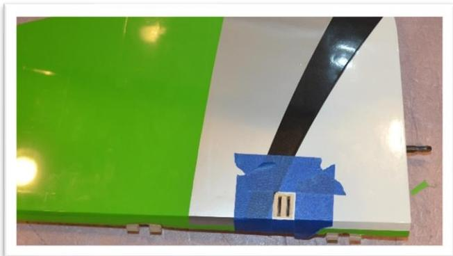
Use sand paper to roughen up the control horns so the epoxy will adhere better. Assemble the control horns with a ball link and brass cable eye. Thread the cable eyes about half way into the ball link.
