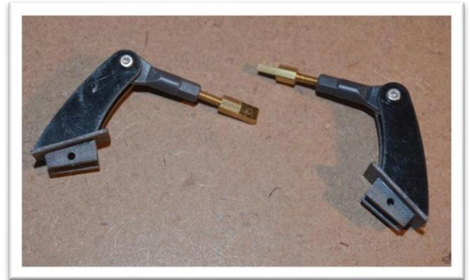
Test fit the control horns to the slots and align with the hinge line. The control horns should be symmetrical about the hinge line.
