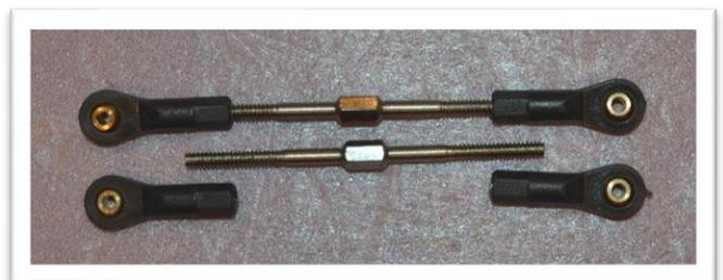
Connect the connecting rod to the servo control arm and the aileron control horn using 2mm machine screws, locking nuts and a flat washer at the servo control arm. (Turn on the transmitter, receiver and servo while making adjusting to the connecting rod. This will keep the servo in its correct position.)
