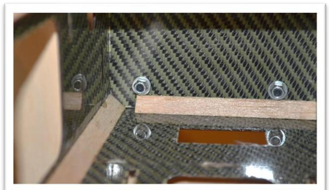
Use an "X" mount with a mounting bolt circle of 75mm to mount your motor. Use the 4mm bolts and washers. Add removable thread locker during installation.
