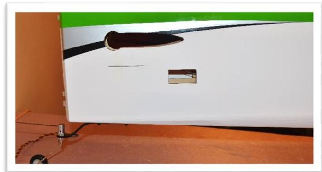
Slide the horizontal stabilizer through the fuselage pushing it all the way forward. Center it side to side.
