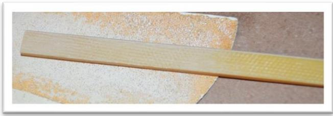
Test fit the elevator jointer plate to each elevator half. Insert the jointer plate into both halves and look down the hinge line. It should be straight. If not use a small file and adjust the slots a little at a time. (Do not glue it yet.)
