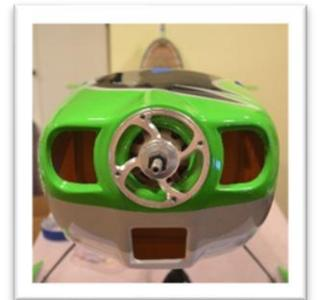
Drill a 1/16" hole in the cowl through the locating holes you created in the tape.
