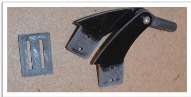
Apply epoxy to the slots in the elevator. Use a pin to help push some epoxy into the slots.
