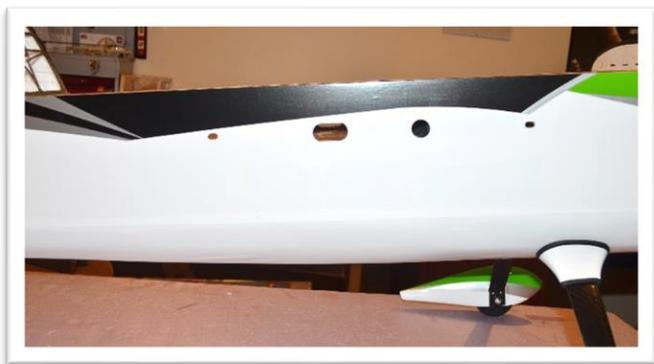
Carefully locate the horizontal stabilizer pocket. Use a trim iron to seal the covering around the edges of the pocket before trimming. Use a new hobby knife blade to cut through the covering.
