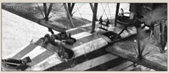
Cockpit coaming detail from converted early production Felixstowe F.2a N4297 B2 . Note the petrol pumps, square hatch for the engineer, Scarff ring on the rear coaming and smaller Scarff ring on the bow.
