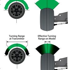
steering sensitivity may be helpful when driving on low-traction surfaces, when driving at high speed, or on tracks that favor sweeping turns where gentle steering inputs are required. The ranges are exaggerated for illustrative purposes.
