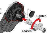
noise. Remove the rubber slipper clutch plug on the transmission cover in order to adjust the slipper. Use the 4-way wrench to turn the adjusting nut clockwise to tighten and counter-clockwise to loosen. Place the model on a high-traction surface, such as carpet. Adjust the slipper so that you can hear it slip for approximately two feet from a standing, full throttle start. (Learn more about adjusting the slipper clutch in the sidebar.)
