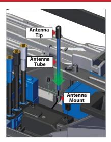
making sure that antenna wire is in the slot in the antenna mount, then install the set screw next to the antenna tube. Use a 1.5mm wrench to tighten the screw just until the antenna tube is securely in place. Do not over tighten. Do not bend or kink the antenna wire! See the sidebar for more information. Do not shorten the antenna tube.
