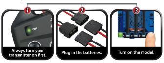
Always use new batteries for the radio system. Weak batteries will limit the radio signal between the receiver and the transmitter. Loss of the radio signal can cause you to lose control of your model.
