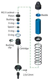
3. Remove the M2.5 locknut, piston, 2.5x5mm washer, and the existing cartridge assembly from the shock shaft.
