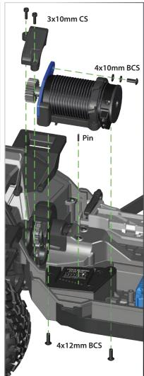
gear. Tighten the two 4x12mm button-head cap screws, and then remove the strip of paper. You should be able to run a fresh strip of paper through the gears without binding them.
