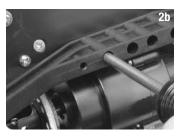
Remove the eight 3x12RM screws located in the chassis braces that secure the transmission to the chassis.
