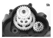
Place the complete single speed gear hub assembly into the transmission case half next to the new slipper shaft. Apply a light coating of grease to the gears (such as Traxxas lithium grease part #5148).
