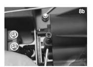
Insert the brake lever into the brake cam and tighten the 3x3GS. Connect the shift linkage back onto the shift fork by popping the rod end onto the ball stud. Install the air filter back onto the carburetor. This completes the single speed installation.
