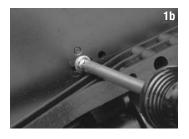
Remove the 3x10WM screw from the bottom of the carb linkage bell crank post. (Models equipped with TRX 2.5 Racing Engine only).
