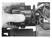
Lift the transmission from the chassis.
