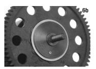
Fit the spur gear over the bushing followed by the second pressure ring and pressure plate.
