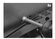
Set the carb linkage bell crank post assembly back onto the chassis (keying the post into the appropriate holes) and secure it with the 3x10WM screw.
