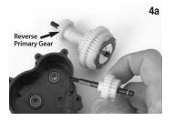
Remove the 2-speed primary gear shaft assembly and the 2-speed slipper shaft (#4992) from the transmission half.
