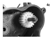
Locate the single speed slipper shaft (#5193) and insert the shaft into the transmission case half where the 2-speed slipper shaft was located.
