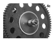
Slide the slipper spring (#1994) over the slipper shaft and secure the assembly with the 4.0NL. Tighten the slipper nut until it stops then back it off 1/4 turn.
