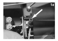
Begin by removing the air filter. Disconnect the shift linkage from the shift fork that exits the front of the transmission. Loosen the 3x3GS on top of the brake cam and remove the brake lever from the brake cam.
