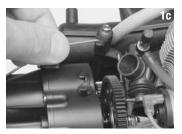
Lift the bell crank assembly off of the chassis (this is to provide access to the transmission).
