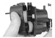
Connect the two transmission halves making sure that all gears and shafts are aligned correctly. Secure the transmission halves with the seven 3x10RST screws.
