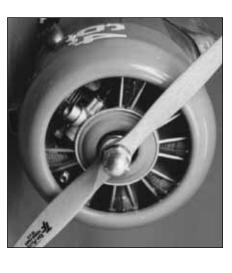
The Top Flite® Dummy Radial Engine (hereafter referred to as *Radial*) is patterned after the Pratt & Whitney radial engines that powered numerous aircraft from the *Golden Age* of aviation. Modeled to fit the Top Flite F4U Corsair and AT-6 Texan, this 1/7th scale Radial will fit any cowls with a frontal opening of 6-1/2" to 7". Not only does the Radial enhance scale appearance, but it also serves as an air-flow baffle for more efficient engine cooling.
