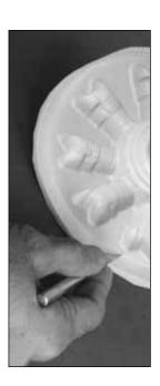
3. Score around the inside comer of the Radial with a hobby knife. Flex the plastic around the rim until it breaks off.
