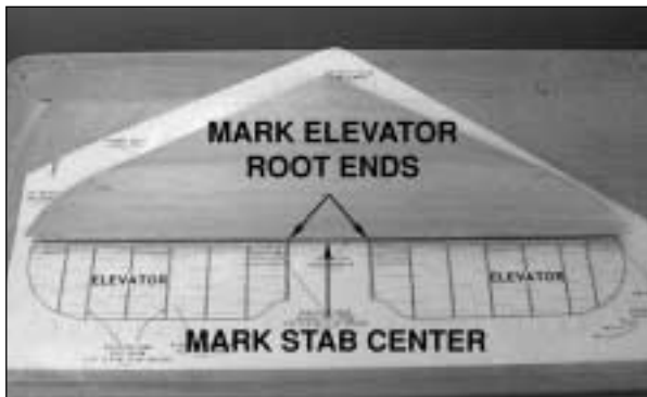
□ 13. Sheet the top of the stab with one of the stab skins you've already prepared. We recommend using aliphatic
