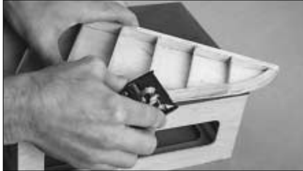
□ 14. Remove the stab from your building board. Save the rib jigs for building your fin. Turn the stab over and cut the jig tabs from the bottom of the ribs, then trim the bottom of the LE even with the ribs. Trim the stab tips and the bottom of the TE near the tips the same way you did on the top. Trim the bottom of the rudder torque rod block even with the ribs.
