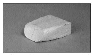
□ 9. Shape the balsa cowl bottom as shown in the photograph. The cross-section of former F-1 also shows the shape of the front of the cowl bottom.
