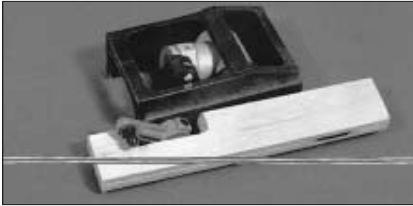
“Photos of Violett T-33 main landing gear and suggested 1/4” plywood aft mounting rail”
