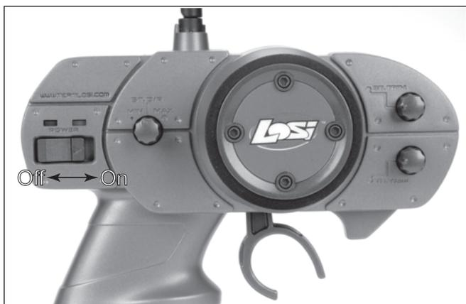
Always turn on the transmitter first. The small red and green lights above the switch should both light up. If not, you need to check for low or incorrectly installed batteries.
