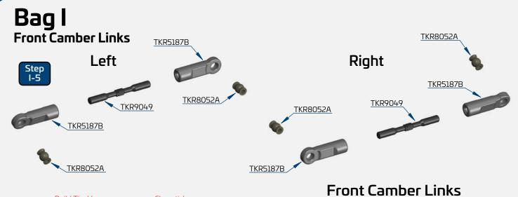
Build Tip: Use some grease or Chapstick on the threads to help prevent "pop-off" when adjustments are being made.
